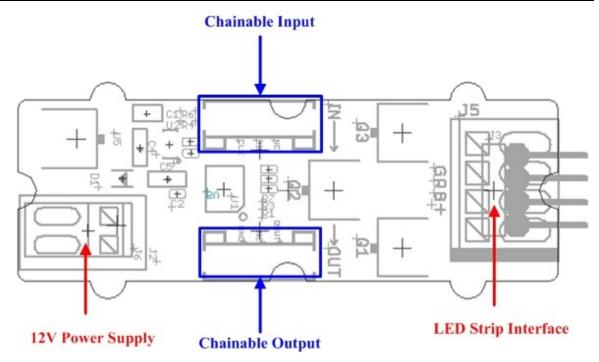
**12V Power Supply** – Screw terminal for 9~12v power supply.
