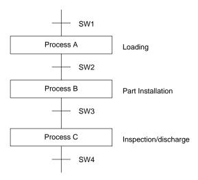
The program for this process, shown below, utilizes the most basic type of step programming: each step is completed by a unique SNXT(09) that starts the next step. Each step starts when the switch that indicates the previous step has been completed turns ON.
