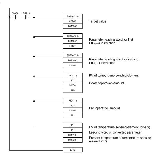
**Note** When using PID(—) or SCL(—), make the data settings in advance with a Peripheral Device such as the Programming Console or LSS.
