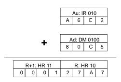
**Note** The UF and OF flags would also be turned ON during this addition, but they can be ignored since they are relevant only in the addition of signed binary data.
