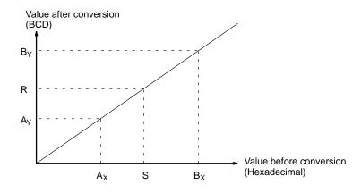
The results can be calculated by first converting all values to BCD and then using the following formula.
