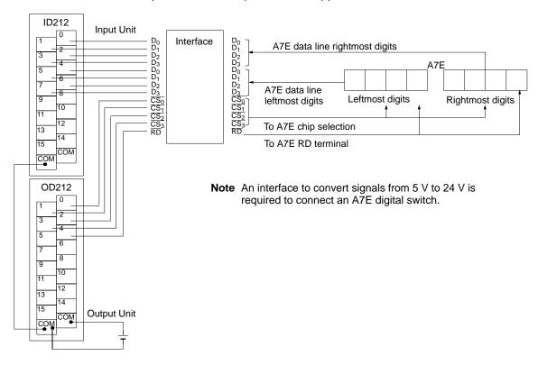
The following example illustrates connections for an A7B Thumbwheel Switch.
