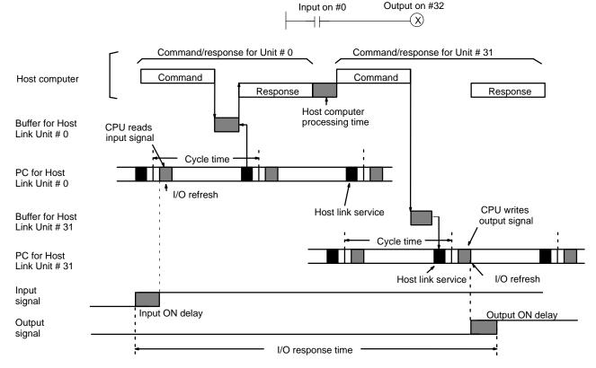
The equations used to calculate the minimum and maximum cycle times are given below. The number of cycles required for each PC depends on the amount of data being read/written.
