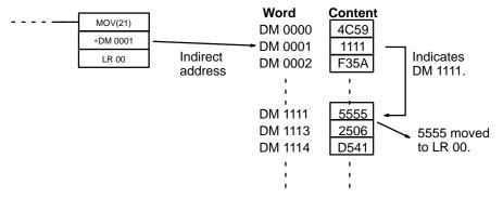
When using indirect addressing, the address of the desired word must be in BCD and it must specify a word within the DM area. In the above example, the content of \*DM 0000 would have to be in BCD between 0000 and 1999.
