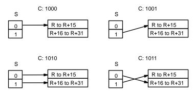
The following is an example of a one-byte decode operation from the rightmost byte of S (C would be 1000 in this case).
