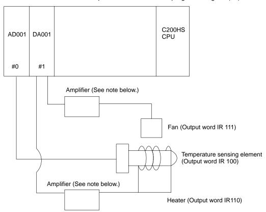
**Note** Motors and heaters cannot be directly connected from a Analog Output Unit. An amplifier (i.e., a current amplification circuit) is required.
