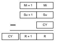
**Note** The DOUBLE 2's COMPLEMENT – NEGL(—) instruction can be used to convert binary data only, it cannot be used with BCD data.
