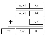
ADBL(—) can also be used to add signed binary data. The underflow and overflow flags (SR 25404 and SR 25405) indicate whether the result has exceeded the lower or upper limits of the 32-bit signed binary data range. Refer to page 29 for details on signed binary data.
