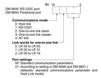
The standard communications parameters are as shown in the following table.
