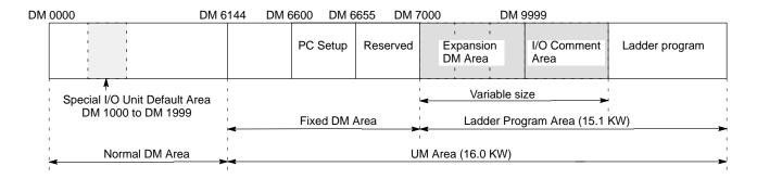
**Note** Allocating UM area for an expansion DM and/or I/O Comment Area will reduce program capacity. Check program capacity requirements before allocating the UM area.
