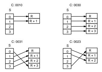
The following is an example of a one-digit decode operation from digit number 1 of S, i.e., here C would be 0001.
