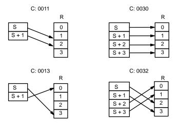
The following is an example of a one-digit encode operation to digit number 1 of R, i.e., here C would be 0001.
