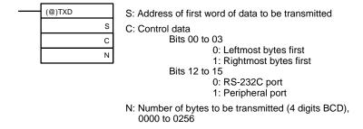
3. From the time this instruction is executed until the data transmission is complete, SR 26405 (or SR 25413 for the peripheral port) will remain OFF. It will turn ON again upon completion of the data transmission.
