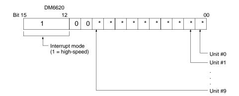
Note Disabling special I/O refreshing in the normal cycle to refresh special I/O in an interrupt subroutine is necessary only in the high-speed mode. Disabling normal cycle refreshing of special I/O during normal interrupt mode will be ignored and the special I/O will be refreshed both in the normal cycle and in the interrupt subroutine.
