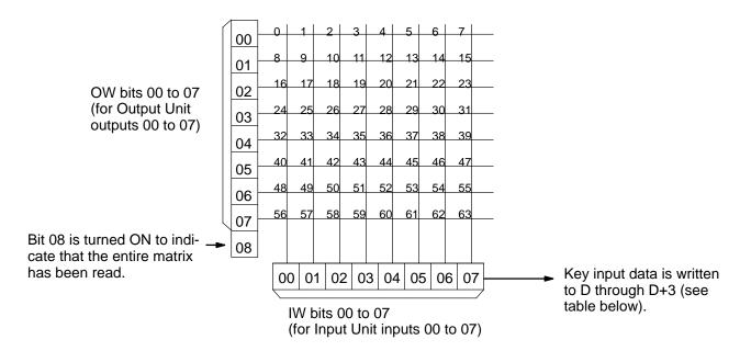
A selection signal is output to OW bits 00 to 07 consecutively for 3 cycles. Only one output bit will be turned on at a time. Bit 08 of OW is turned ON for 3 cycles after 07 to indicate when each round of reading the matrix has been completed.
