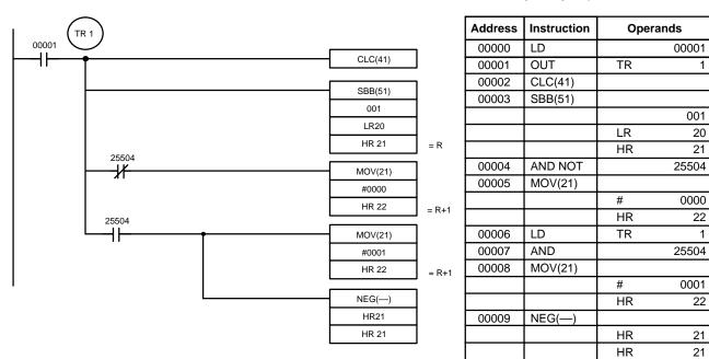
In the case below, the content of LR 20 (#7A03) and CY are subtracted from IR 001 (#F8C5). The result is stored in HR 21 and the content of HR 22 (#0000) indicates that the result is positive.
