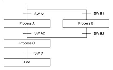
The program for this process, shown below, starts with two SNXT(09) instructions that start processes A and B. Because of the way 00001 (SW A1) and 00002 (SB B1) are programmed, only one of these will be executed to start either process A or process B. Both of the steps for these processes end with a SNXT(09) that starts the step for process C.
