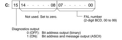
Logic Diagnostic Instructions If the time until the logic diagnostics condition goes ON exceeds T, the logic diagnostic instructions are searched for the OFF input condition. If more than one input condition is OFF, the input condition on the highest instruction line and nearest the left bus bar is selected.
