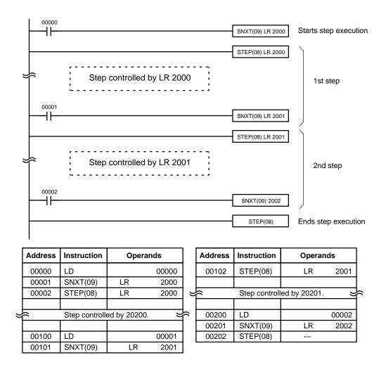
Steps can be programmed in consecutively. Each step must start with STEP(08) and generally ends with SNXT(09) (see example 3, below, for an exception). When steps are programmed in series, three types of execution are possible: sequential, branching, or parallel. The execution conditions for, and the positioning of, SNXT(09) determine how the steps are executed. The three examples given below demonstrate these three types of step execution.
