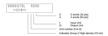
**Note** Group-2 HIgh-density I/O Units will not be displayed in the I/O table when it is displayed using LSS (host computer). Four asterisks (\*\*\*\*), indicating no Unit, will be displayed instead.
