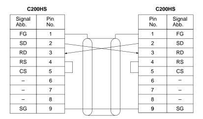
**Note** Ground the FG terminals the C200HS to a resistance of 100  $\Omega$  or less.
