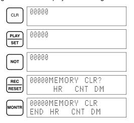
**Note** When the write-protect switch (pin 1 of the CPU's DIP switch) is set to ON the UM area (from DM 6144 through the ladder program) will not be cleared. Other data areas, such as HR, AR, CNT, and DM from DM 0000 to DM 6143 will be cleared.
