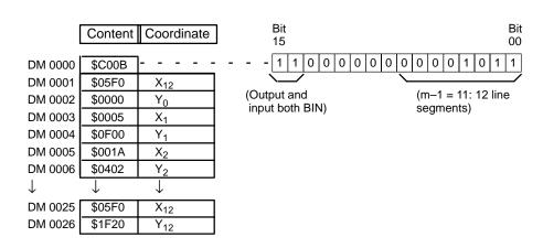
In this case, the input data word, IR 010, contains #0014, and f(0014) = #0726 is output to R, IR 011.
