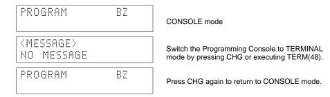
Expansion TERMINAL Mode The Programming Console can be put into Expansion TERMINAL mode by turning ON AR 0709. Pin 6 of the CPU's DIP switch must be ON.
