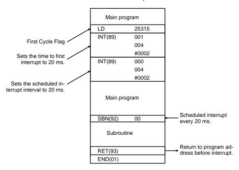
**Note** Depending on the setting of DM 6621 in the PC Setup, Host Link servicing, Remote I/O servicing, Special I/O Unit servicing, and individual instruction execution will be completed before the subroutine is executed. Refer to page 255 for details.
