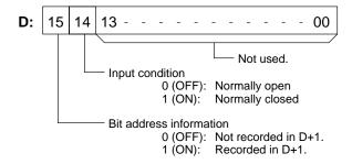
> D+1 contains the bit address code of the input condition, as shown below. The word addresses, bit numbers, and TC numbers are in binary.
