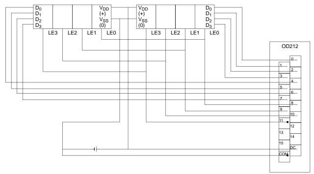
The outputs must be connected from an Output Unit with 8 or more output points for four digits or 16 or more output points for eight digits. Basic Output, Special I/O, or High-density Output Units can be used.
