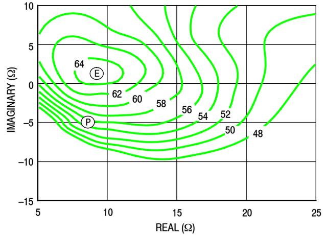
Figure 18. P1dB Load Pull Efficiency Contours (%)
