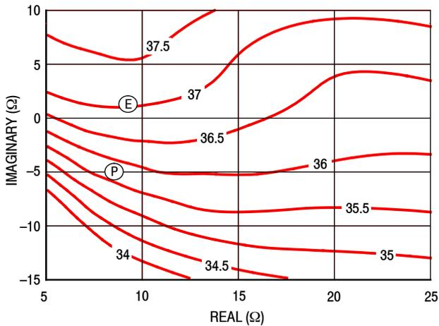
Figure 19. P1dB Load Pull Gain Contours (dB)
