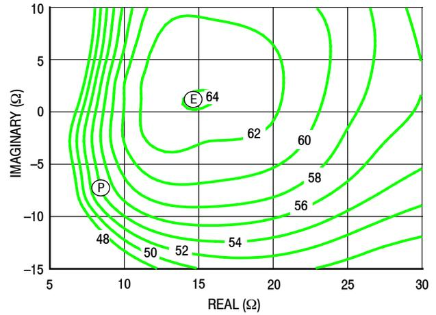
Figure 14. P3dB Load Pull Efficiency Contours (%)
