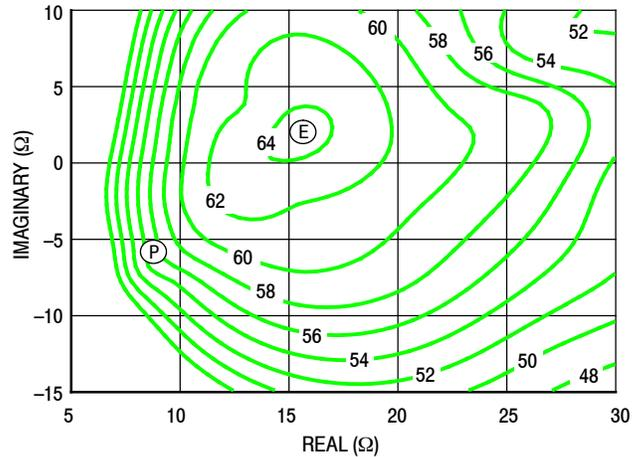
Figure 10. P1dB Load Pull Efficiency Contours (%)
