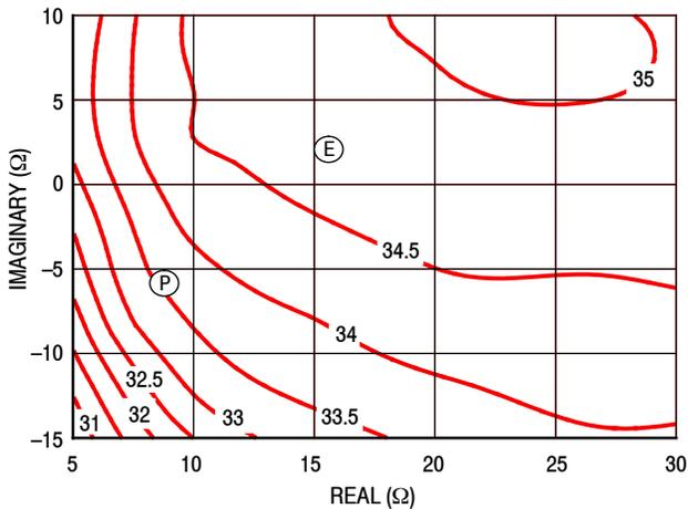
Figure 11. P1dB Load Pull Gain Contours (dB)
