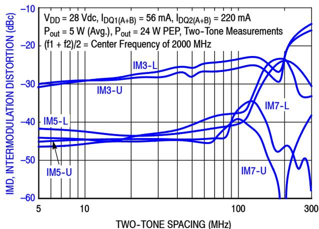
**Figure 5. Intermodulation Distortion Products versus Two-Tone Spacing**
