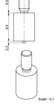
Technical Tolerances according to DIN ISO 2768m In tape & reel packaging a cap is fixed to the product to realize automatic assembly
