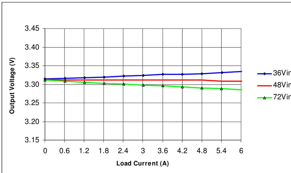
Figure 3. Regulation – Note regulation band of 1.5%
