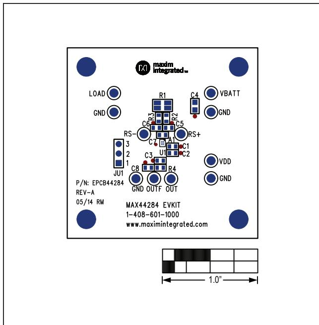
Figure 2. MAX44284 EV Kit Component Placement Guide—Component Side
