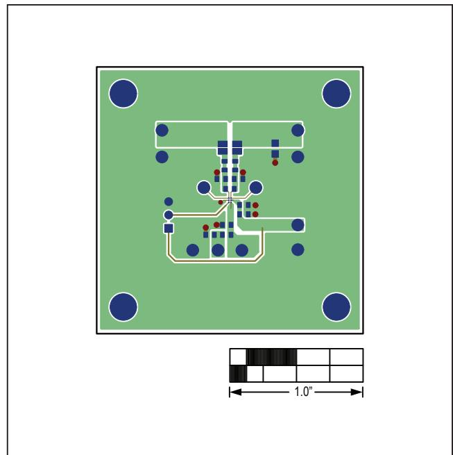
Figure 3. MAX44284 EV Kit PCB Layout—Component Side
