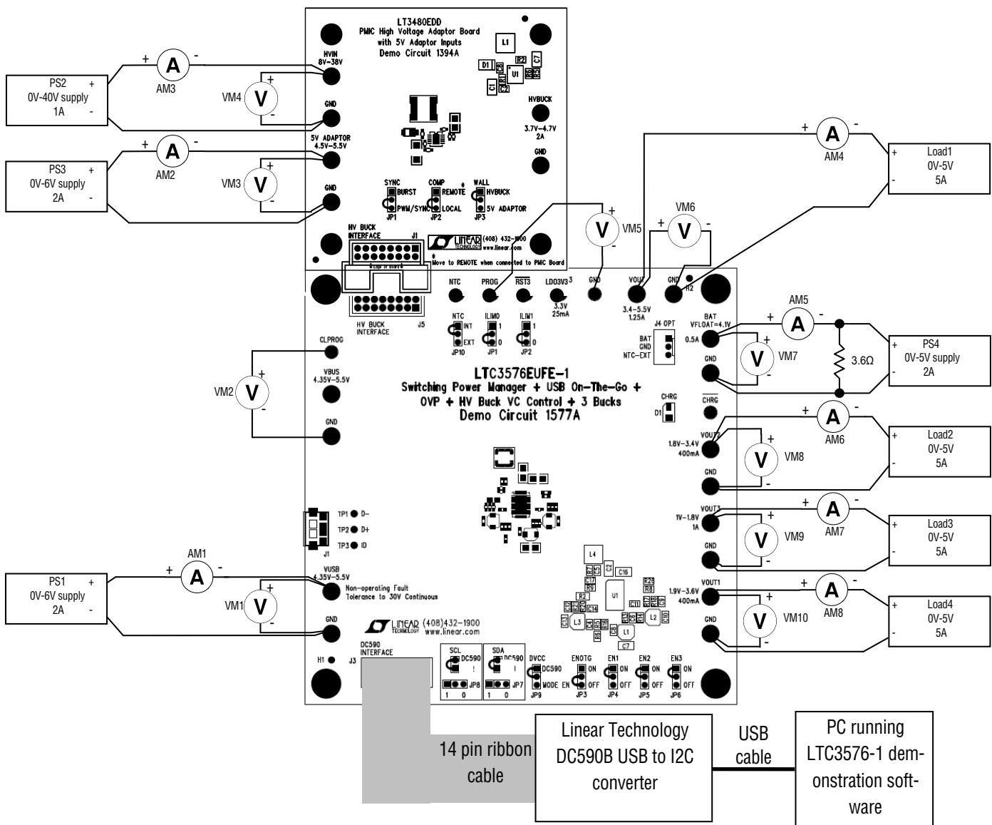
Note: All connections from equipment should be Kelvin connected directly to the Board PINS which they are connected to on this diagram and any input, or output, leads should be twisted pair
