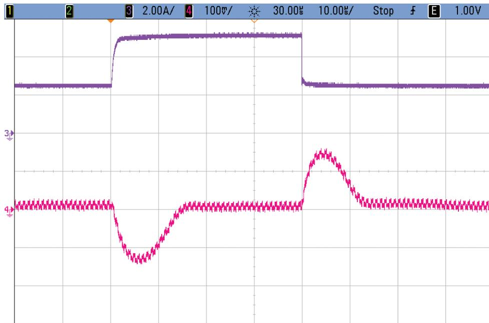
Figure 4. Transient Response Waveform at 12V<sub>IN</sub>, 5V<sub>OUT</sub> and 2.5 – 5 – 2.5A<sub>OUT</sub> (2A, 100mV, 10μs/DIV, 20MHz Bandwidth)
