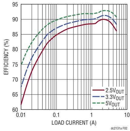
Figure 2. 12V<sub>IN</sub> DCM Efficiency
