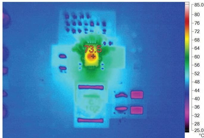
Figure 5. Thermal at 12V<sub>IN</sub>, 3.3V<sub>OUT</sub> and 5A<sub>OUT</sub>, OLFM
