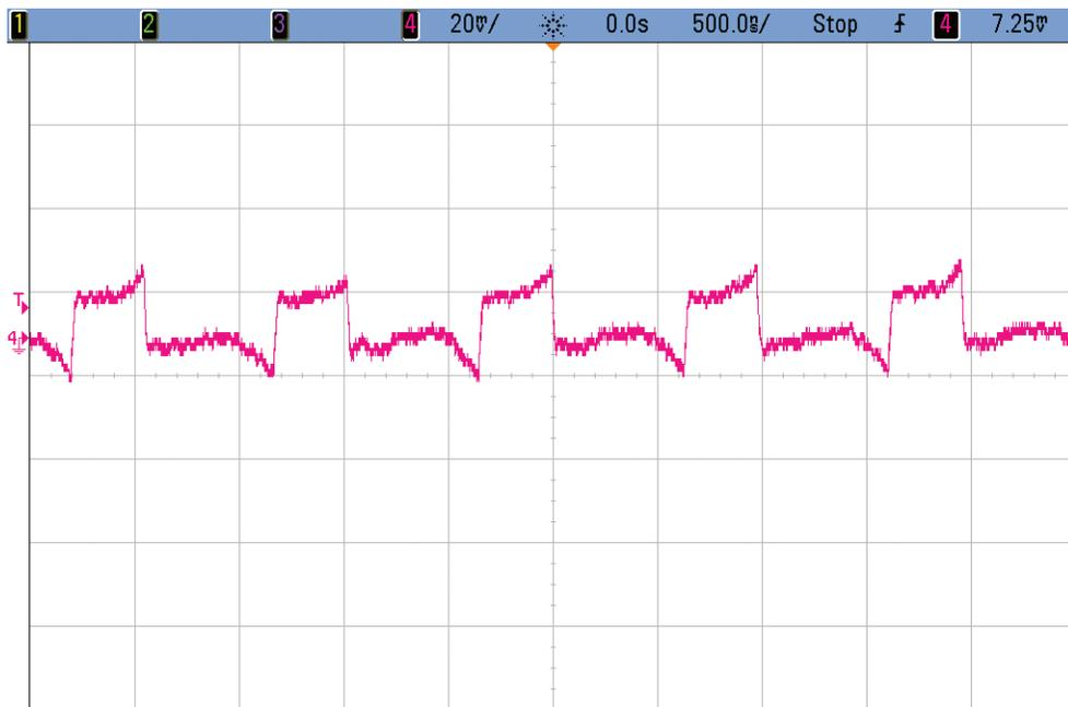
Figure 3. Output Ripple at 15V<sub>IN</sub>, 5V<sub>OUT</sub> and 5A<sub>OUT</sub> (20mV, 500ns/DIV, 20MHz Bandwidth)
