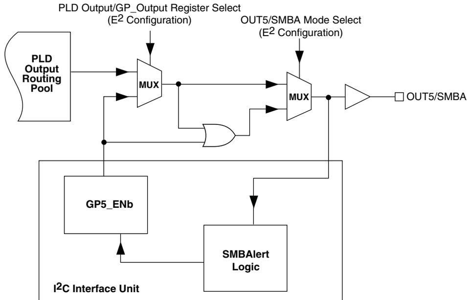
The typical flow for an SMBAlert transaction is as follows (Figure 31):
