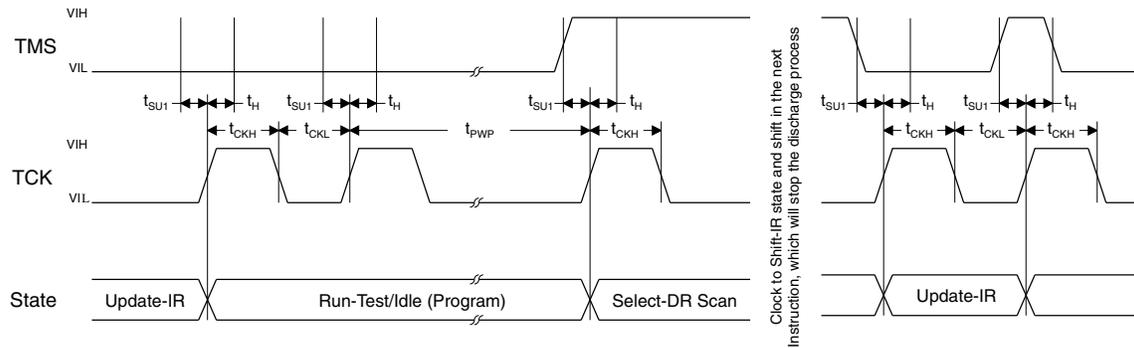
Figure 5. Verify Timing Diagram
