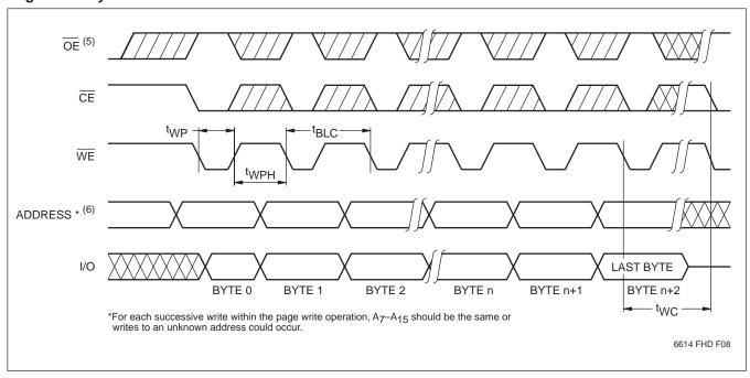
Notes: (5) Between successive byte writes within a page write operation,  $\overline{OE}$  can be strobed LOW: e.g. this can be done with  $\overline{CE}$  and  $\overline{WE}$  HIGH to fetch data from another memory device within the system for the next write; or with  $\overline{WE}$  HIGH and  $\overline{CE}$  LOW effectively performing a polling operation.
