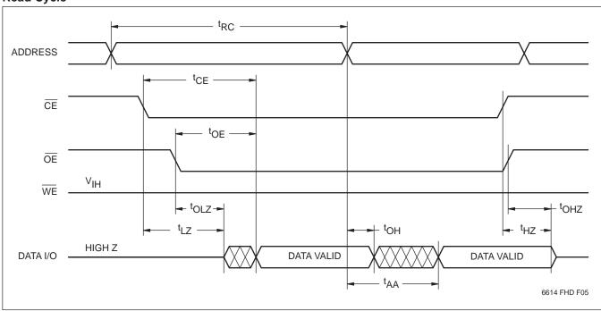
Notes: (3)  $t_{LZ}$  min.,  $t_{HZ}$ ,  $t_{OLZ}$  min., and  $t_{OHZ}$  are periodically sampled and not 100% tested.  $t_{HZ}$  max. and  $t_{OHZ}$  max. are measured, with  $C_L = 5pF$  from the point when  $\overline{CE}$  or  $\overline{OE}$  return HIGH (whichever occurs first) to the time when the outputs are no longer driven.
