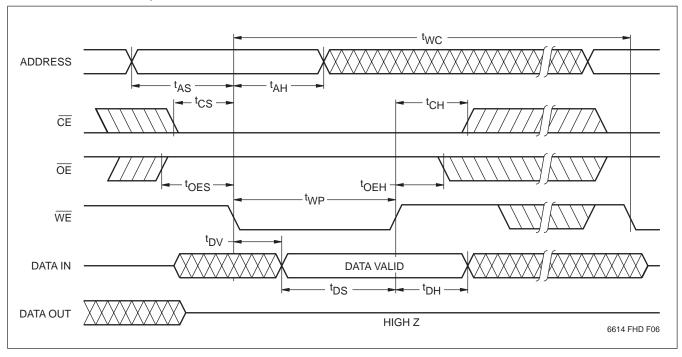
Notes: (4) t<sub>WC</sub> is the minimum cycle time to be allowed from the system perspective unless polling techniques are used. It is the maximum time the device requires to complete the internal write operation.
