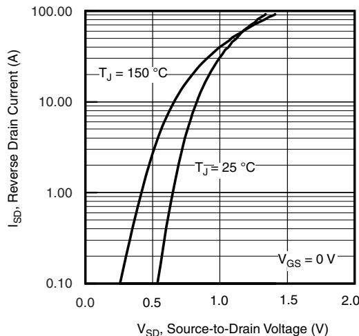
**Fig. 9 - Typical Source-Drain Diode Forward Voltage**
