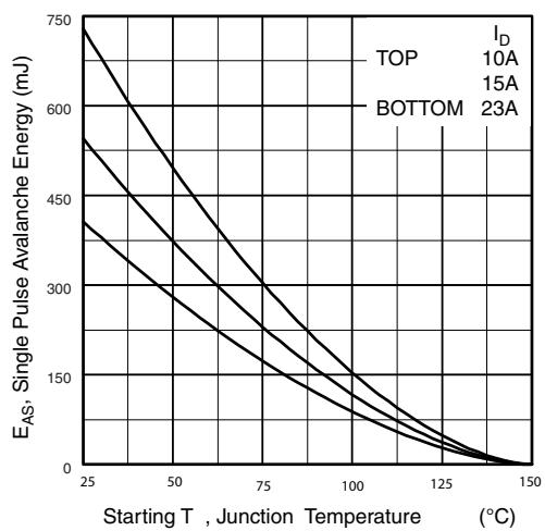
Fig. 14 - Maximum Avalanche Energy s. Drain Current
