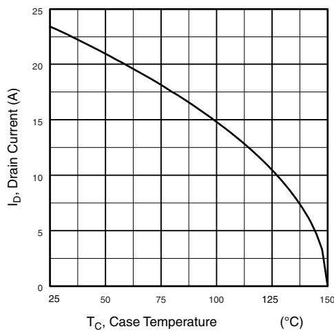
**Fig. 10 - Maximum Drain Current vs. Case Temperature**
