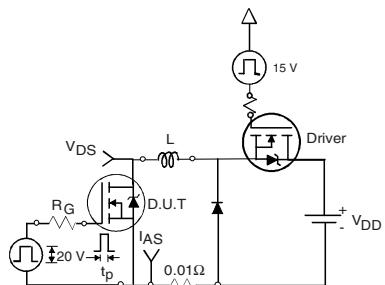
Fig. 15a - Unclamped Inductive Test Circuit
