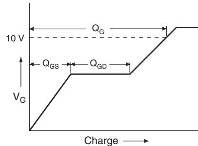
Fig. 16b - Basic Gate Charge Waveform
