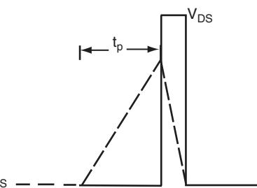
Fig. 15b - Unclamped Inductive Waveforms
