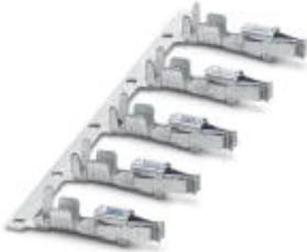
Module socket contact, inserted in the PCC or HCC plug housing after crimping the conductor, for 1.5 mm<sup>2</sup> ... 2.5 mm<sup>2</sup> conductors, ribbon contact
