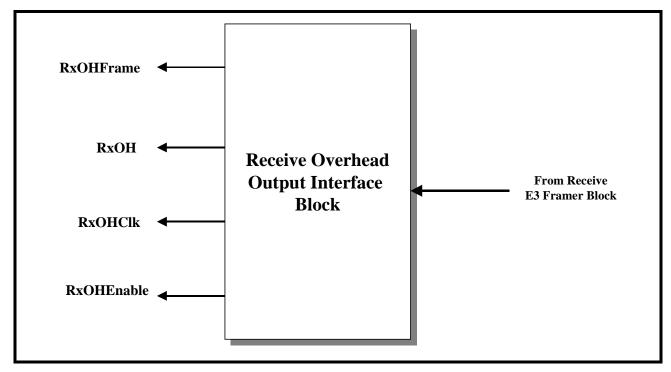
The E3, ITU-T G.751 frame consists of 1536 bits. Of these bytes, 1524 bits are payload bits and the remaining 12 bits are overhead bits. The XRT72L53 has been designed to handle and process both the payload type and overhead type bits for each E3 frame.
