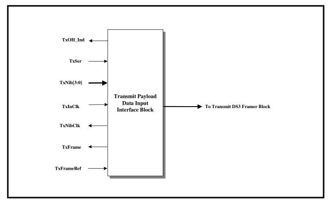
Each of the input and output pins of the Transmit Payload Data Input Interface are listed in Table 19 and described below. The exact role that each of these
