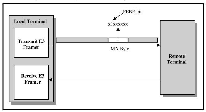
In additional to the FEBE bit-field signaling, the Receive E3 Framer block will generate the BIP-8 Error Interrupt to the Microprocessor. Hence, it will set bit 2
