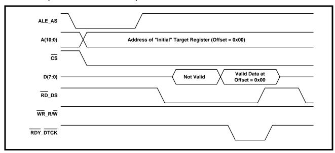
At the completion of this initial read cycle, the  $\mu$ C/ $\mu$ P has read in the contents of the first register or buffer location (within the XRT72L53 DS3/E3 Framer) for this particular burst access operation. In order to illustrate how this burst I/O cycle works, the byte (or word) of data, that is being read in Figure 33 has been la-
