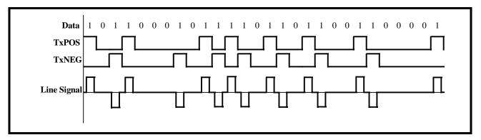
**Note:** One of the main reasons that the AMI Line Code has been chosen for driving transformer-coupled media is that this line code introduces no dc component, thereby minimizing dc distortion in the line.
