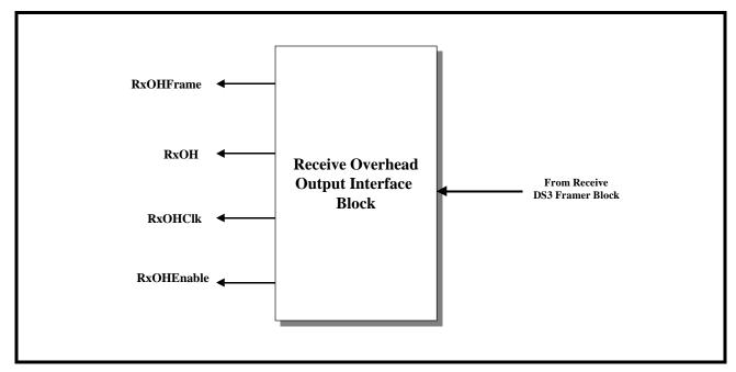
The DS3 frame consists of 4760 bits. Of these bits, 4704 bits are payload bits and the remaining 56 bits are overhead bits. The XRT72L53 has been designed to handle and process both the payload type and overhead type bits for each DS3 frame.
