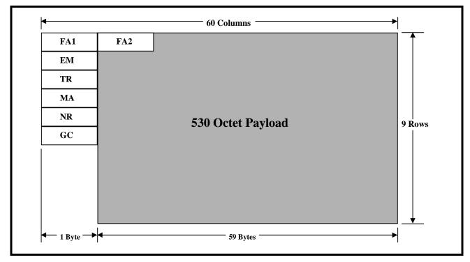
When the Receive E3 Framer block detects the "FA1" octet, and determines that this octet is immediately followed by the "FA2" octet, then it will transition to the FA1, FA2 Octet Verification state, per Figure 195.
