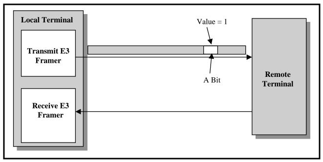
In additional to the FEBE bit-field signaling, the Receive E3 Framer block will generate the BIP-4 Error Interrupt to the Microprocessor. Hence, it will set bit 2
