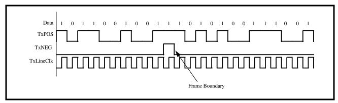
When the Transmit E3 LIU Interface block is operating in the Bipolar (or Dual Rail) mode, then the contents of the E3 Frame is output via both the TxPOS and Tx-NEG pins. If the Bipolar mode is chosen, then E3 data can be transmitted to the LIU via one of two differ-
