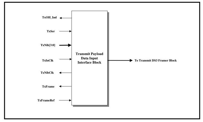
Each of the input and output pins of the Transmit Payload Data Input Interface are listed in Table 47 and described below. The exact role that each of these in-
