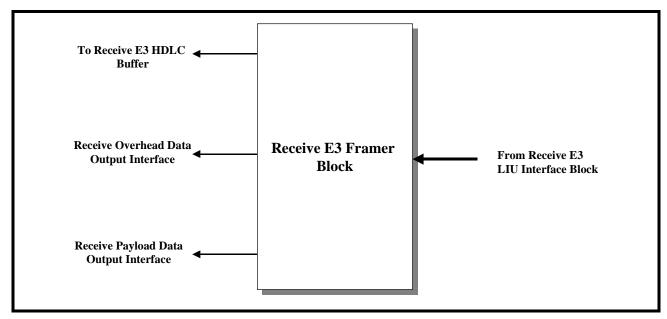
Once the HDB3 (or AMI) encoded data has been decoded into a binary data-stream, the Receive E3 Framer block will use portions of this data-stream in order to synchronize itself to the remote terminal equipment. At any given time, the Receive E3 Framer block will be operating in one of two modes.
