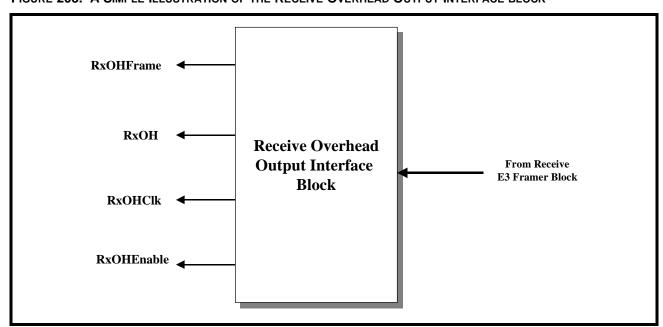
The E3, ITU-T G.832 frame consists of 537 bytes. Of these bytes, 530 bytes are payload bits and the remaining 7 bytes are overhead bytes. The XRT72L53
