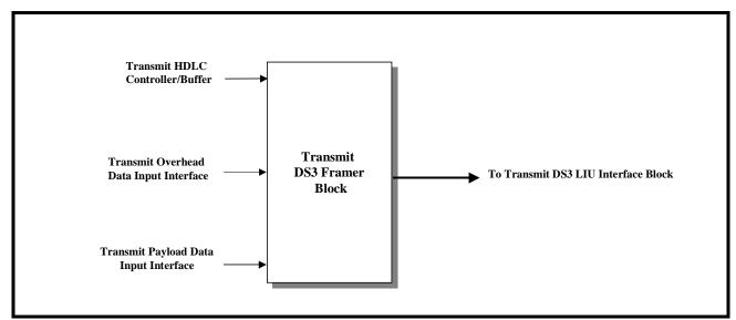
In addition to taking data from multiple sources and multiplexing them, in appropriate manner, to create the outbound DS3 frames, the Transmit DS3 Framer block has the following roles.
