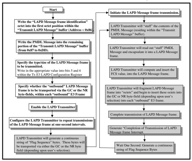
Figure 176 presents the procedure (in white boxes) which the user should use in order to transmit a PM-DL Message via the LAPD Transmitter, when the
