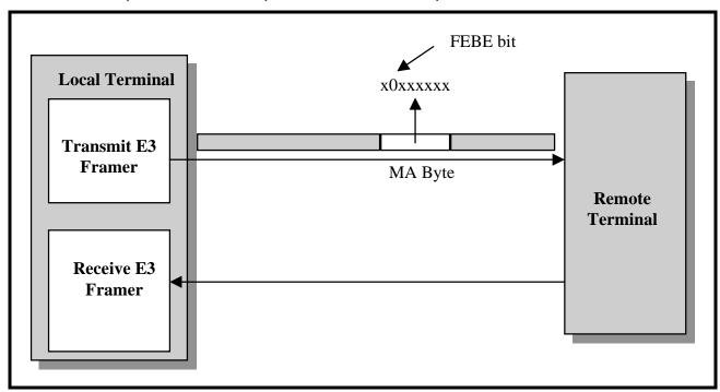
However, if the locally computed BIP-8 value does not match the EM byte of the corresponding E3 frame, then the Receive E3 Framer block will do the following.
