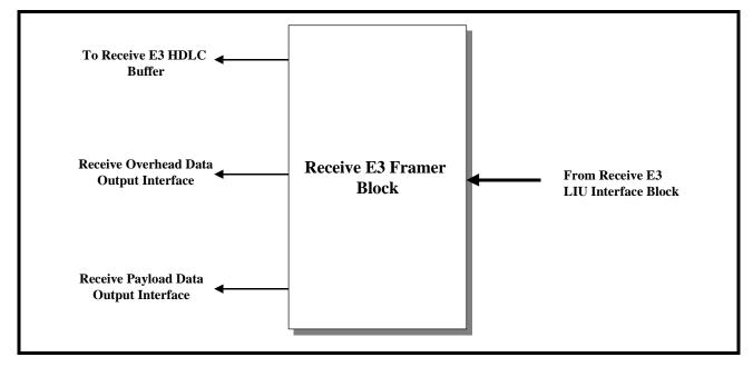
Once the HDB3 (or AMI) encoded data has been decoded into a binary data-stream, the Receive E3 Framer block will use portions of this data-stream in order to synchronize itself to the remote terminal equipment. At any given time, the Receive E3 Framer block will be operating in one of two modes.
