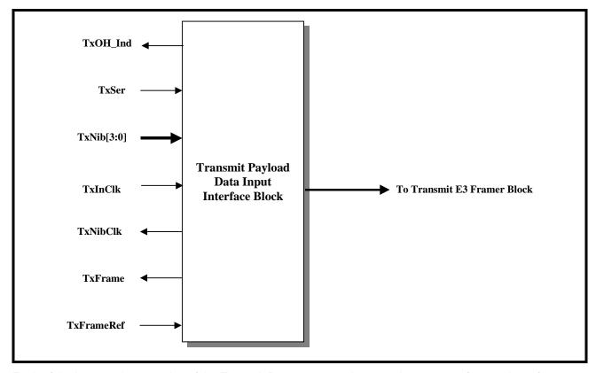
Each of the input and output pins of the Transmit Payload Data Input Interface are listed in Table 71 and described below. The exact role that each of these in-
