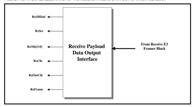
Each of the output pins of the Receive Payload Data Output Interface block are listed in Table 68 and described below. The exact role that each of these output pins assume, for a variety of operating scenarios are described throughout this section.
