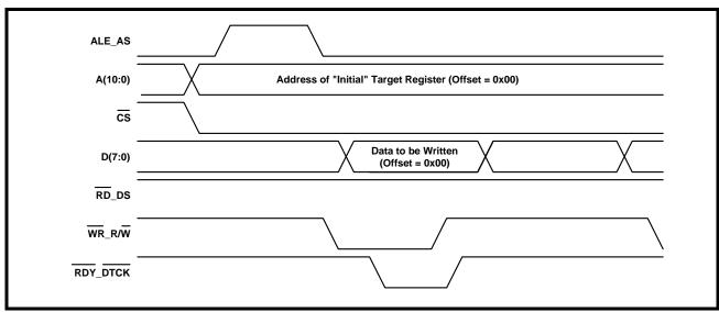
At the completion of this initial write cycle, the  $\mu C/\mu P$  has written a byte or word into the first register or buffer location (within the XRT72L53 DS3/E3 Framer) for this particular burst access operation. In order to
