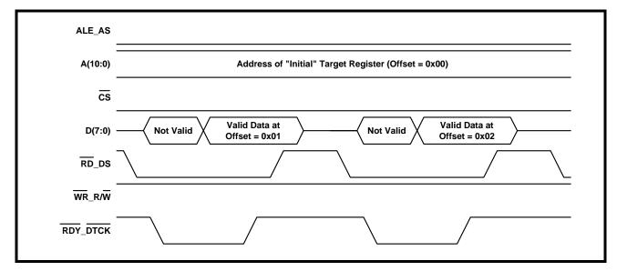
In addition to the behavior of the Microprocessor Interface signals, Figure 30 also illustrates other points regarding the Burst Access Operation.
