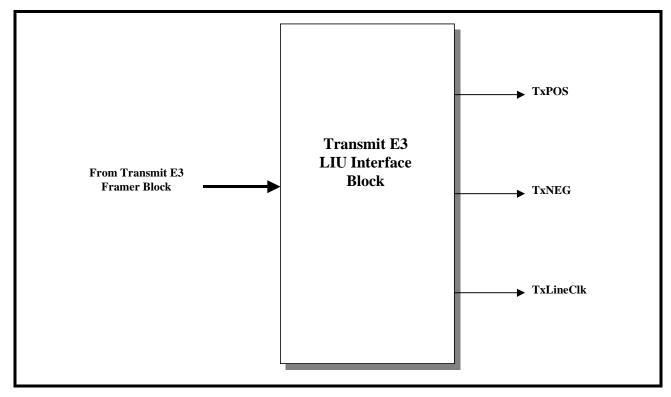
The Transmit E3 LIU Interface block can transmit data to the LIU IC or other external circuitry via two different output modes: Unipolar or Bipolar. If the user selects Unipolar (or Single Rail) mode, then the contents of the E3 Frame is output, in a binary (NRZ manner) data stream via the TxPOS pin to the LIU IC. The TxNEG pin will only be used to denote the frame boundaries. TxNEG will pulse "High" for one bit peri-
