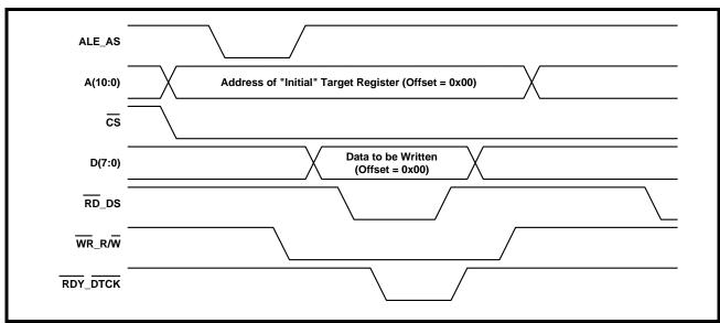
At the completion of this initial write cycle, the µC/µP has written a byte or word into the first register or buffer location (within the XRT72L53 DS3/E3 Framer) for this particular burst I/O access. In order to illustrate how this burst I/O cycle works, the byte (or word) of data, that is being written in Figure 35 has been labeled Data to be Written (Offset = 0x00).
