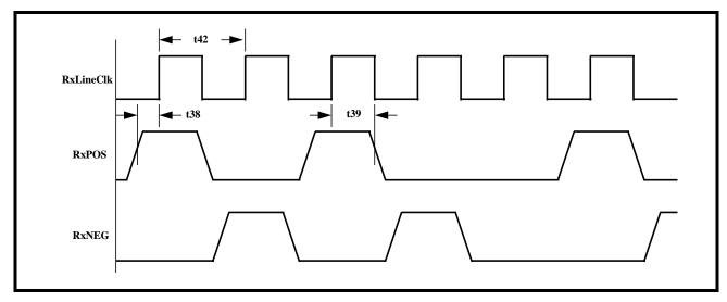
FIGURE 192. WAVEFORM/TIMING RELATIONSHIP BETWEEN RXLINECLK, RXPOS AND RXNEG - WHEN RXPOS AND RXNEG ARE TO BE SAMPLED ON THE FALLING EDGE OF RXLINECLK
