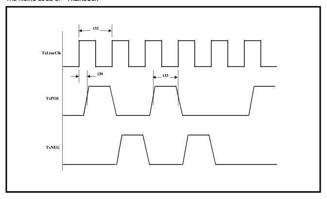
FIGURE 10. TRANSMIT LIU INTERFACE TIMING - FRAMER IS CONFIGURED TO UPDATE "TXPOS" AND "TXNEG" ON THE FALLING EDGE OF "TXLINECLK"
