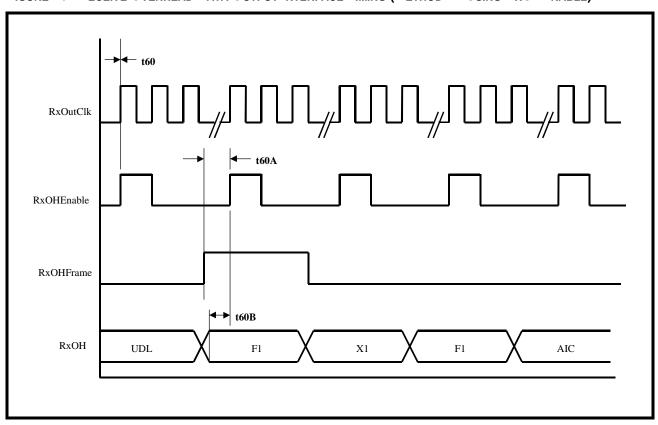
FIGURE 17. MICROPROCESSOR INTERFACE TIMING - INTEL TYPE PROGRAMMED I/O READ OPERATIONS
