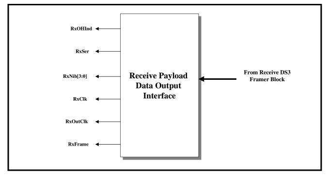
Each of the output pins of the Receive Payload Data Output Interface block are listed in Table 46 and described below. The exact role that each of these output pins assume, for a variety of operating scenarios are described throughout this section.
