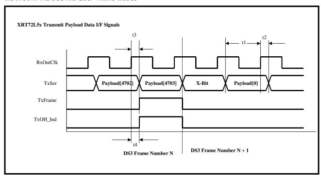
FIGURE 4. TIMING DIAGRAM FOR THE TRANSMIT PAYLOAD INPUT INTERFACE, WHEN THE XRT72L53 DEVICE IS OPERATING IN BOTH THE DS3 AND LOCAL-TIMING MODES
