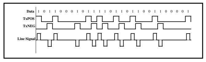
**Note:** One of the main reasons that the AMI Line Code has been chosen for driving transformer-coupled media is that this line code introduces no dc component, thereby minimizing dc distortion in the line.
