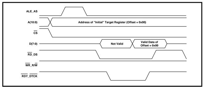
At the completion of this initial read cycle, the  $\mu C/\mu P$  has read in the contents of the first register or buffer location (within the XRT72L53 DS3/E3 Framer) for this particular burst I/O access operation. In order to illustrate how this burst access operation works, the byte (or word) of data, that is being read in Figure 29, has been labeled Valid Data at Offset = "0x00". This
