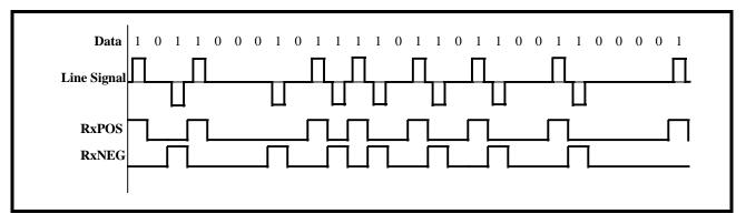
**Note:** One of the reasons that the AMI Line Code has been chosen for driving copper medium, isolated via transformers, is that this line code has no dc component, thereby eliminating dc distortion in the line.
