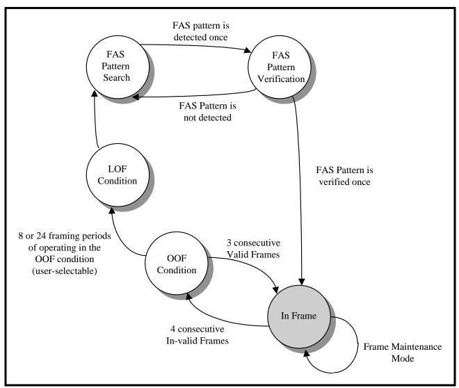
FIGURE 137. ILLUSTRATION OF THE E3, ITU-T G.751 FRAMING FORMAT
