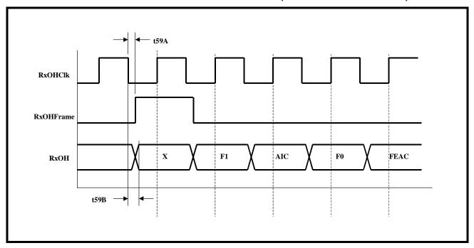
FIGURE 16. RECEIVE OVERHEAD DATA OUTPUT INTERFACE TIMING (METHOD 2 - USING RXOHENABLE)
