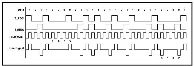
The user chooses between AMI or HDB3 line coding by writing to bit 4 of the I/O Control Register (Address = 0x01), as shown below.
