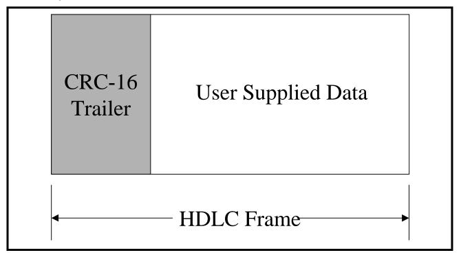
Once the outbound HDLC frame has been formed, then it will be transmitted to the remote terminal equipment via payload bits of the outbound DS3 or E3 frames.
