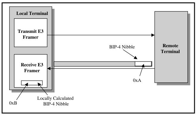
FIGURE 141. ILLUSTRATION OF THE LOCAL RECEIVE E3 FRAMER BLOCK, TRANSMITTING AN E3 FRAME (TO THE REMOTE TERMINAL) WITH THE "A" BIT-FIELD SET TO "1"
