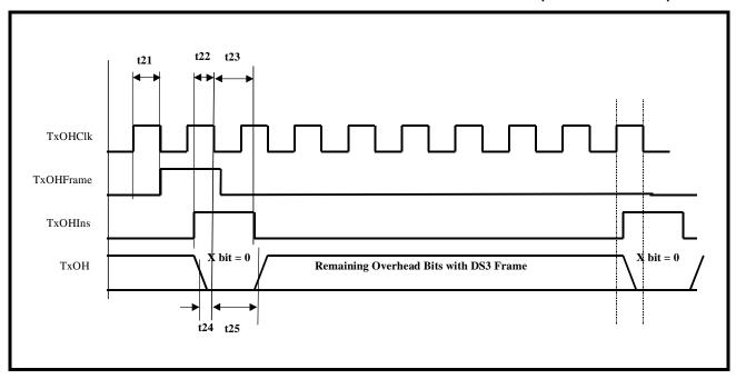
FIGURE 8. TIMING DIAGRAM FOR THE TRANSMIT OVERHEAD DATA INPUT INTERFACE (METHOD 2 ACCESS)
