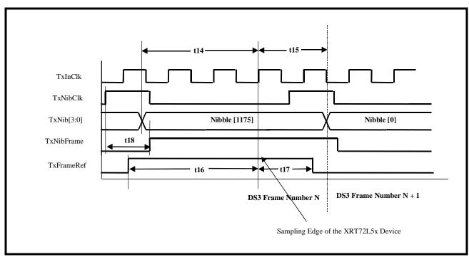
FIGURE 7. TIMING DIAGRAM FOR THE TRANSMIT OVERHEAD DATA INPUT INTERFACE (METHOD 1 ACCESS)
