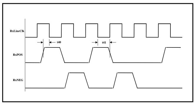
FIGURE 12. RECEIVER LIU INTERFACE TIMING - FRAMER IS CONFIGURED TO SAMPLE "RXPOS" AND "RXNEG" ON THE FALLING EDGE OF "RXLINECLK"
