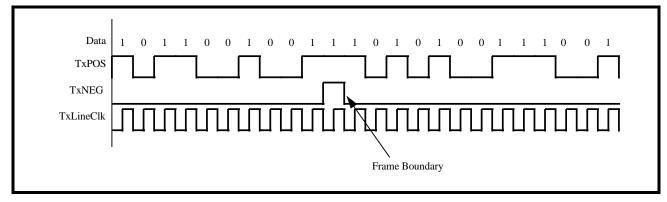
When the Transmit E3 LIU Interface block is operating in the Bipolar (or Dual Rail) mode, then the contents of the E3 Frame is output via both the TxPOS and Tx-NEG pins. If the Bipolar mode is chosen, then the E3
