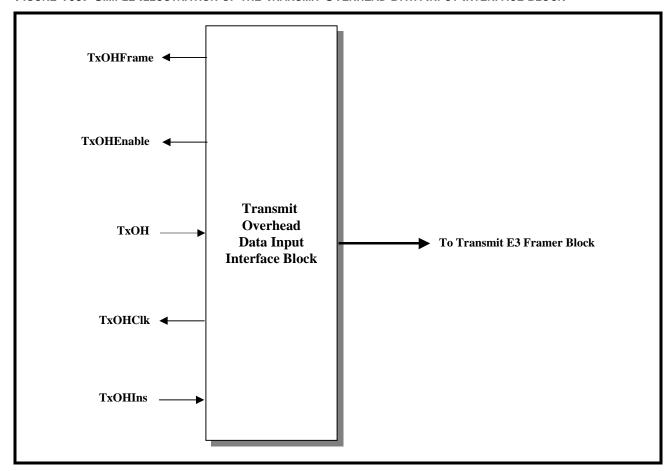
The E3, ITU-T G.832 Frame consists of 537 bytes. Of these bytes, 530 bytes are payload bytes and the remaining 7 are overhead bytes. The XRT72L53 has been designed to handle and process both the payload type and overhead type bits for each E3 frame. Within the Transmit Section within the XRT72L53, the Transmit Payload Data Input Interface has been designed to handle the payload data. Likewise, the Transmit Overhead Input Interface has been designed to handle and process the overhead bits.
