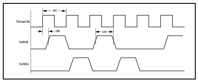
FIGURE 126. WAVEFORM/TIMING RELATIONSHIP BETWEEN TXLINECLK, TXPOS AND TXNEG - TXPOS AND TXNEG ARE CONFIGURED TO BE UPDATED ON THE FALLING EDGE OF TXLINECLK
