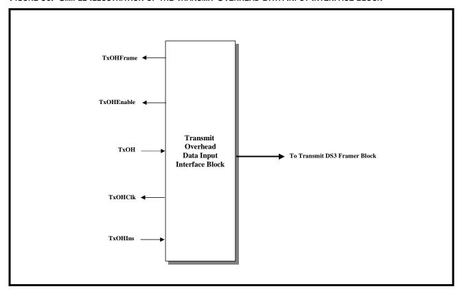
The DS3 Frame consists of 4760 bits. Of these bits, 4704 bits are payload bits and the remaining 56 bits are overhead bits. The XRT72L53 has been designed to handle and process both the payload type and overhead type bits for each DS3 frame. Within the Transmit Section within the XRT72L53, the Transmit Payload Data Input Interface has been designed to handle the payload data. Likewise, the Transmit Overhead Data Input Interface has been designed to handle and process the overhead bits.
