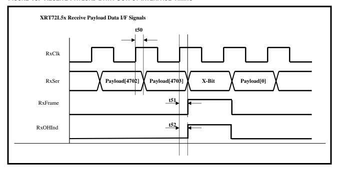
FIGURE 14. RECEIVE PAYLOAD DATA OUTPUT INTERFACE TIMING (NIBBLE MODE OPERATION)
