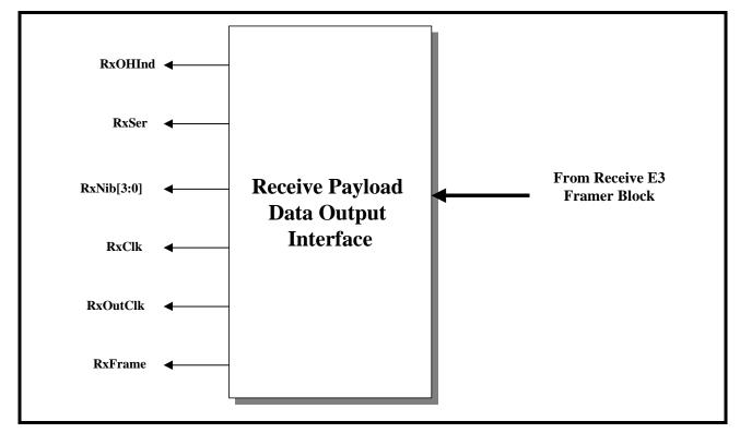
Each of the output pins of the Receive Payload Data Output Interface block are listed in Table 92 and described below. The exact role that each of these output pins assume, for a variety of operating scenarios are described throughout this section.
