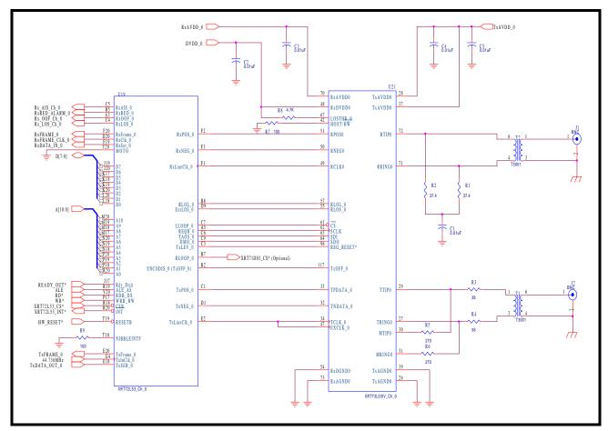
The Transmit Section of the XRT72L53 contains a block which is known as the Transmit E3 LIU Interface block. The purpose of the Transmit E3 LIU Interface block is to take the outbound E3 data stream, from the Transmit E3 Framer block, and to do the following:
