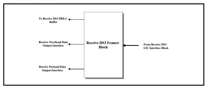
Once the B3ZS (or AMI) encoded data has been decoded into a binary data-stream, the Receive DS3 Framer block will use portions of this data-stream in order to synchronize itself to the remote terminal equipment. At any given time, the Receive DS3 Framer block will be operating in one of two modes.
