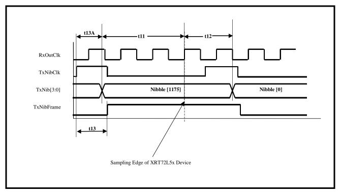
FIGURE 6. TIMING DIAGRAM FOR THE TRANSMIT PAYLOAD DATA INPUT INTERFACE, WHEN THE XRT72L53 DEVICE IS OPERATING IN THE DS3/NIBBLE AND LOCAL-TIMING MODES
