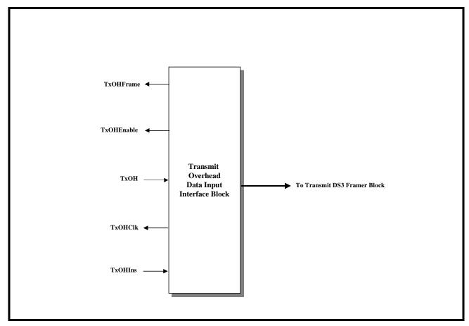
The E3, ITU-T G.751 Frame consists of 1536 bits. Of these bits, 1524 are payload bits and the remaining 12 are overhead bits. The XRT72L53 has been designed to handle and process both the payload type and overhead type bits for each E3 frame. Within the Transmit Section within the XRT72L53, the Transmit Payload Data Input Interface has been designed to handle the payload data. Likewise, the Transmit Overhead Input Interface has been designed to handle and process the overhead bits.
