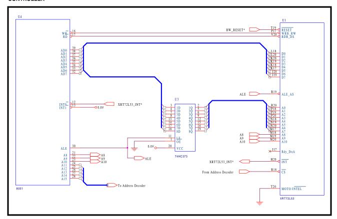
The circuitry in Figure 37 will function as follows, during a Framer-request interrupt. The Framer would request an interrupt from the CPU by asserting its ac-
