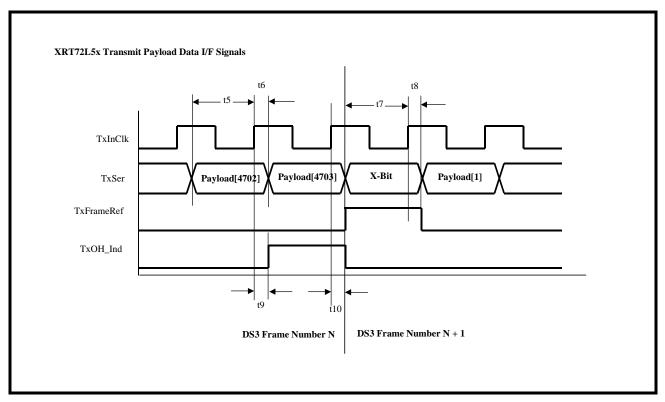
FIGURE 5. TIMING DIAGRAM FOR THE TRANSMIT PAYLOAD DATA INPUT INTERFACE, WHEN THE XRT72L53 DEVICE IS OPERATING IN BOTH THE DS3/NIBBLE AND LOOPED-TIMING MODES
