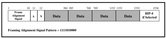
When the Receive E3 Framer block detects the FAS pattern, it will then transition over to the FAS Pattern Verification state, per Figure 137.
