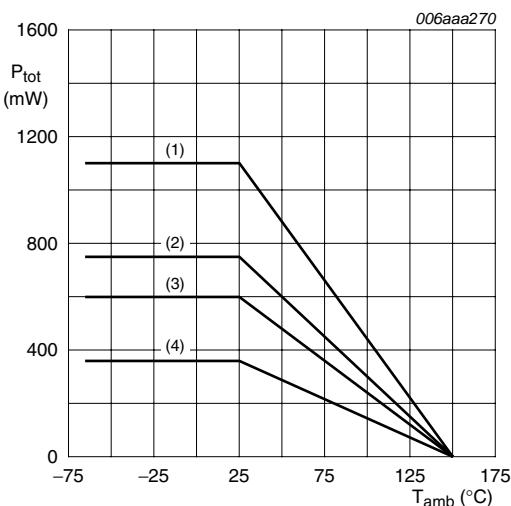
(1) Ceramic PCB,  $Al_2O_3$ , standard footprint(2) FR4 PCB, mounting pad for collector  $6\text{ cm}^2$ (3) FR4 PCB, mounting pad for collector  $1\text{ cm}^2$
