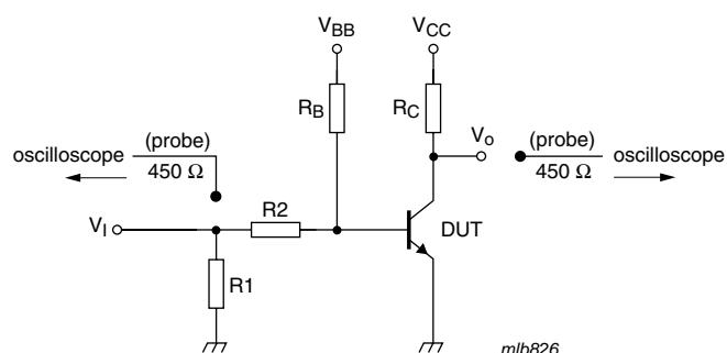
(1)  $V_{CC} = 10$  V;  $I_C = 2$  A;  $I_{Bon} = 0.1$  A;  $I_{Boff} = -0.1$  A
