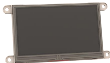
GEN4 4D CAPE 4.3" Resistive Touch Display
