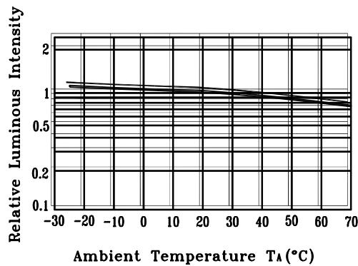
Fig.5 Luminous Intensity vs.
