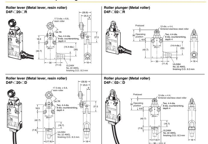
Note: Each dimension has a tolerance of 0.4 mm unless otherwise specified.
