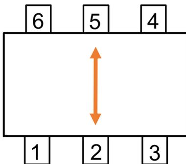
The arrow represent the axis of sensitivity of the two sensors inside the device (as referenced as Rout in Figure 1) that have their axis of sensitivity 180 degrees out of phase with each other.
