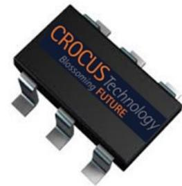
The CT219 provides design flexibility with high sensitivity in a small footprint SOT-26 package and is cost competitive for high volume manufacturing. The CTD203 development board demonstrating the closed-loop circuit solution is available for additional support and guidance.
