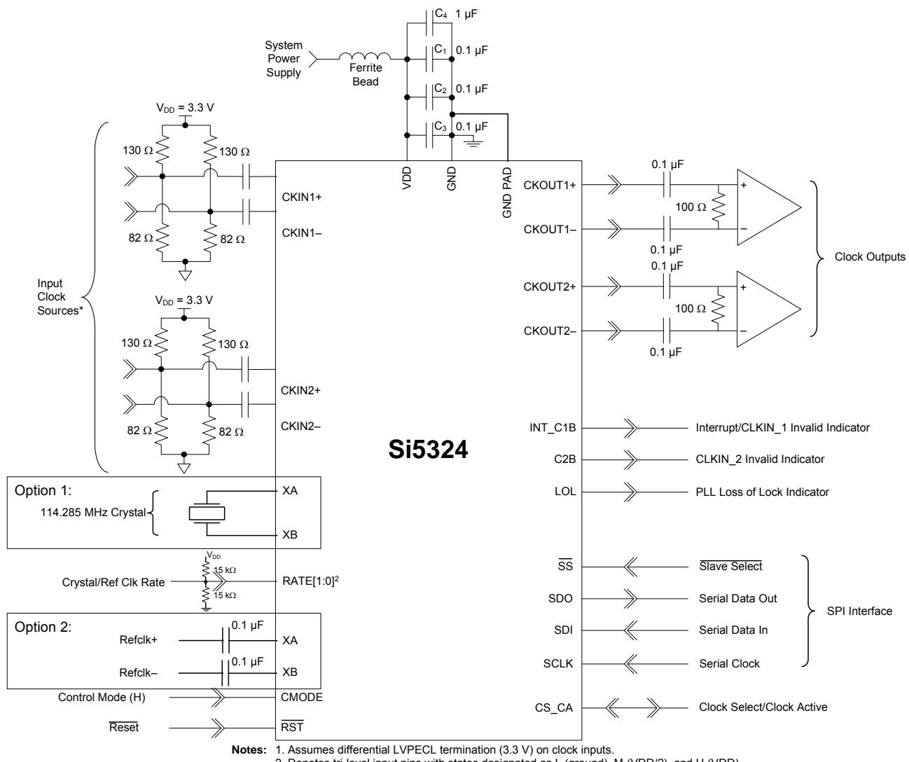
Figure 4. Si5324 Typical Application Circuit (SPI Control Mode)
