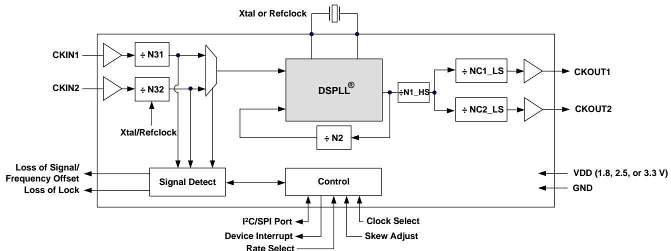
**Figure 5. Si5324 Functional Block Diagram**
