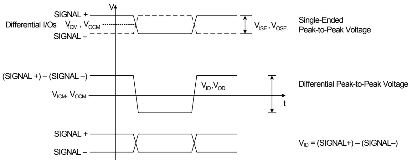
**Figure 1. Differential Voltage Characteristics**
