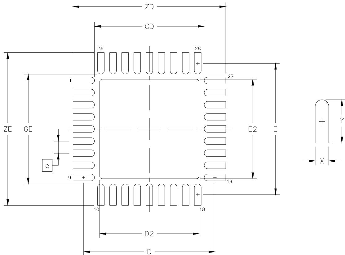
Figure 10. PCB Land Pattern Diagram
