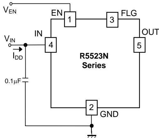
Supply Current Test Circuit
