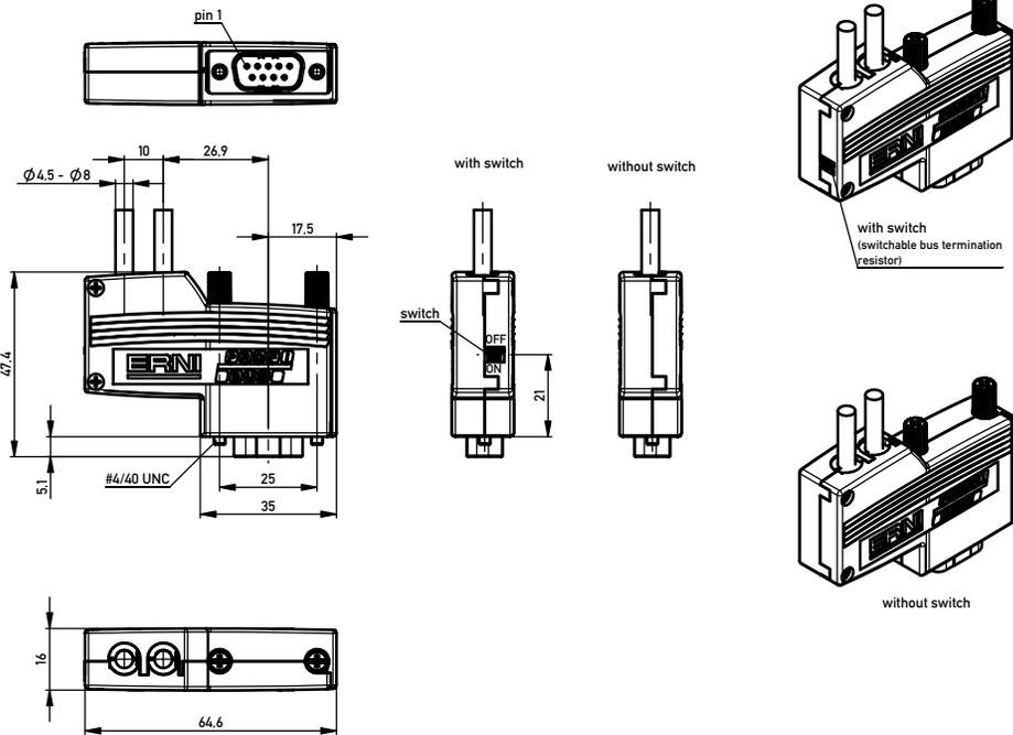
ERbic Profibus with PU interface, vertical
