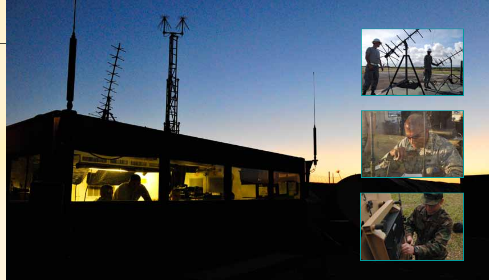
Main Photo: Command and control specialists work inside a Mobile Air Reporting Communications shelter at Camp Marmal, Afghanistan. The MARC is an air-deployable mobile tactical shelter that provides CRW Airmen with the ability to communicate with aircraft as well as schedule and track cargo movements worldwide. Inset Photos: Mobile tactical shelter specialists installing rooftop antennae, working inside a shelter, and checking communications equipment.
