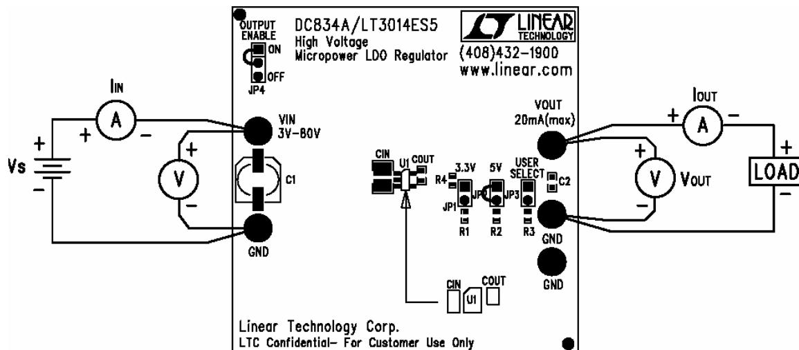
Figure 1. Proper Measurement Equipment Setup
