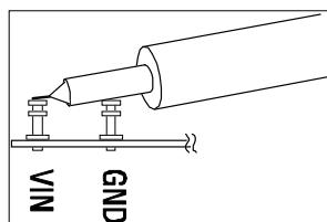
Figure 2. Measuring Input or Output Voltage Ripple
