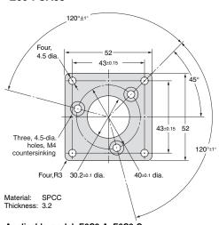
Applicable model: E6C3-A, E6C3-C Note: Three phillips screws M4  $\times$  8 provided
