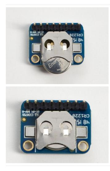
Don't forget that the Real Time Clock requires a battery backup. A CR1220 size battery goes in the back, make sure the + symbol on the battery is visible when you insert!
