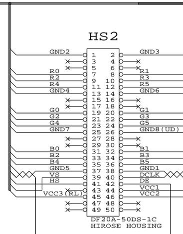
CABLE: UL20276, 17 PAIRS, 30AWG (BRAID SHIELD TYPE), PVC COLOR BLACK, COLOR CODED
