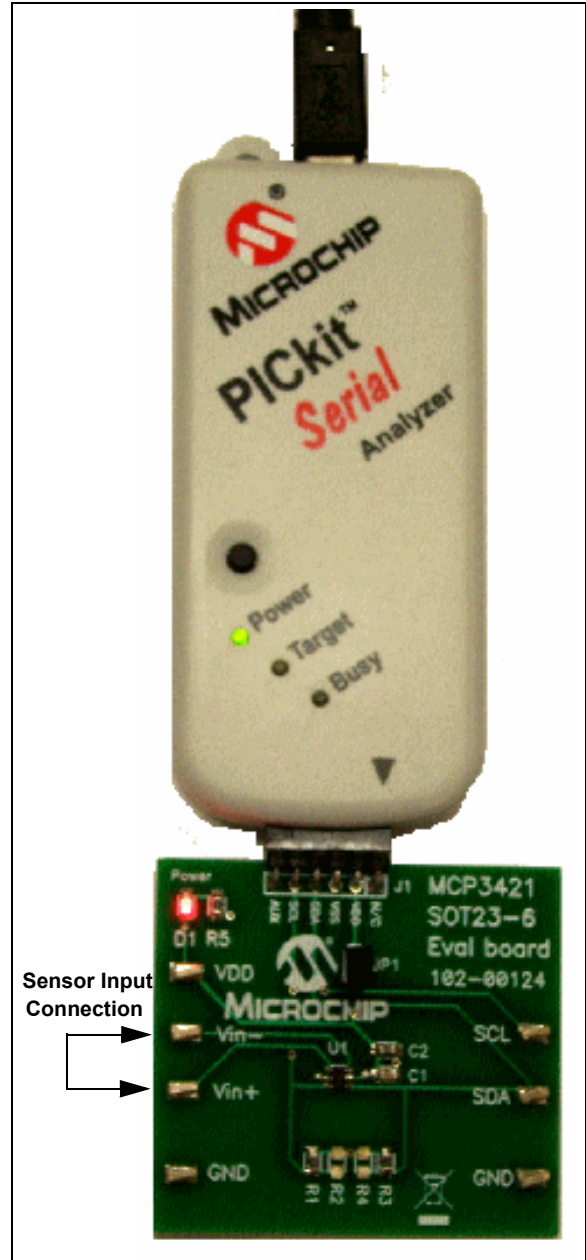
FIGURE 7-2: Setup for the MCP3421 Evaluation Board with PICkit™ Serial Analyzer.
