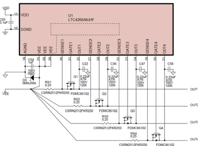
Figure 3. LTC4266A Key Application Components for Board Placement
