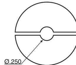
Note: To fit a .250 hole with slot
