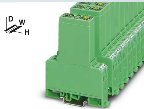
Solid-state power relay Max. 2 A
