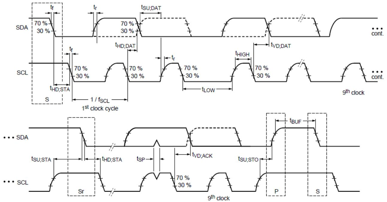
Figure 2. I<sup>2</sup>C Serial Port Timing Standard and Fast Modes
