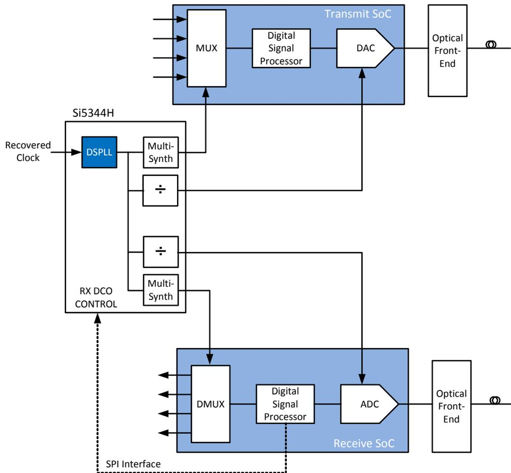
Figure 1. 100G/400G Coherent Optical Transceiver Application Example
