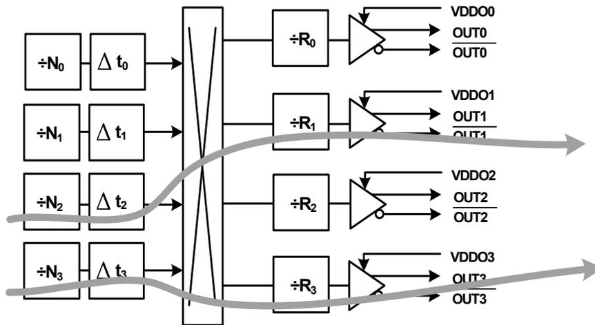
**Figure 23. Example of Independently Configurable Path Delays**
