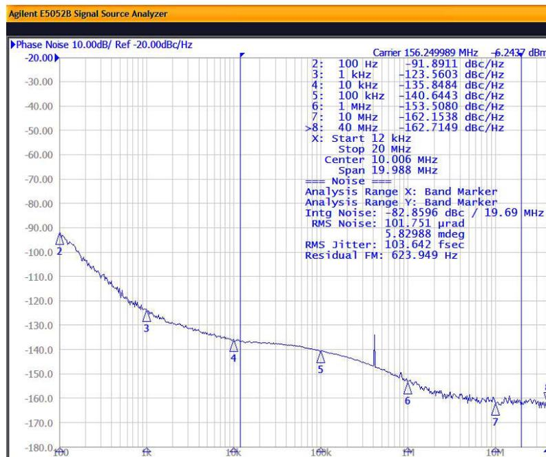
Figure 6. Input = 25 MHz; Output = 156.25 MHz, 3.3 V LVPECL
