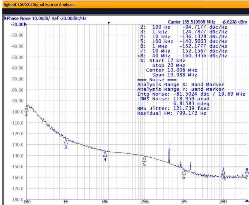
Figure 7. Input = 25 MHz; Output = 155.52 MHz, 3.3 V LVPECL
