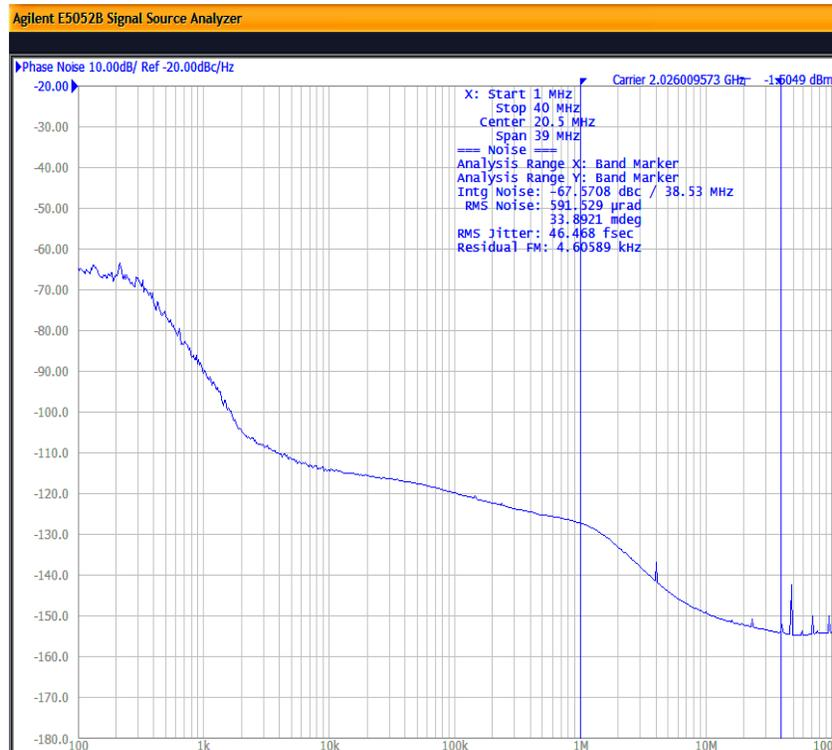
Figure 5. Input = 19.44 MHz; Output = 2.026 GHz, 3.3 V LVPECL
