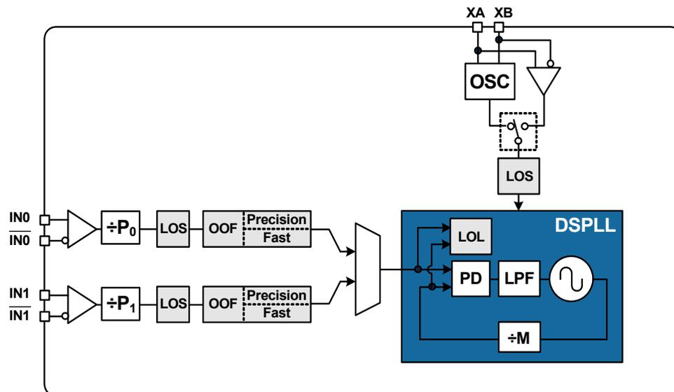
**Figure 14. Fault Monitors**
