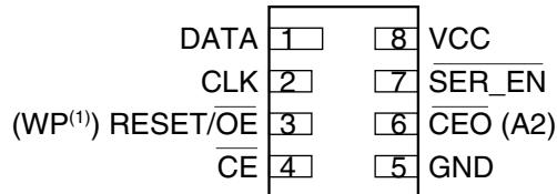
**Figure 2-2.** 8-lead SOIC
