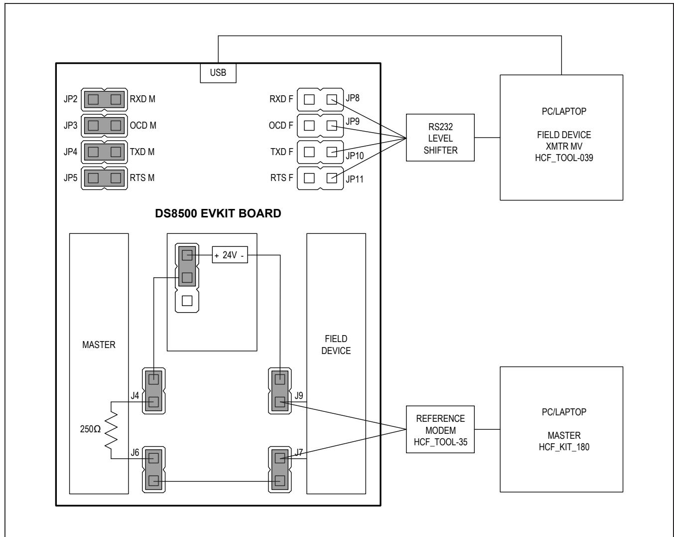
Figure 3. Setup for Emulated Field Device Evaluation
