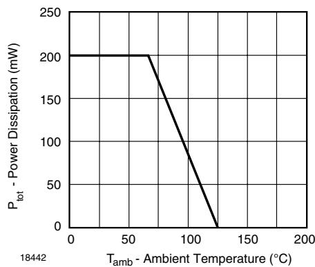
Figure 1. Admissible Power Dissipation vs. Ambient Temperature
