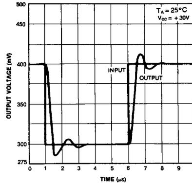
Figure 8. Voltage Follower Pulse Response (Small Signal)
