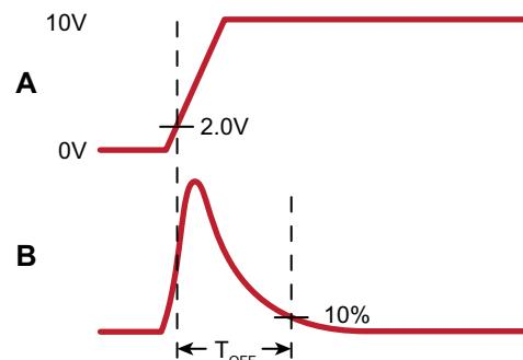
Figure 1:  $T_{OFF}$  Test Circuit
