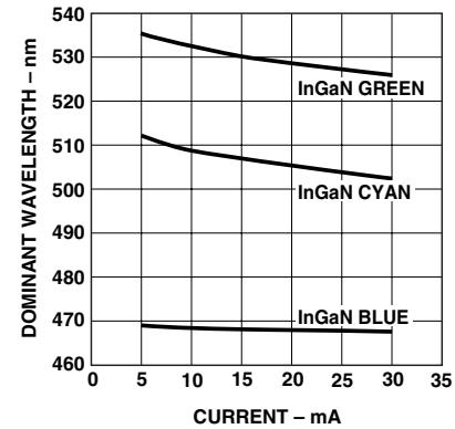
**Figure 6. Dominant wavelength vs. forward current – InGaN devices**
