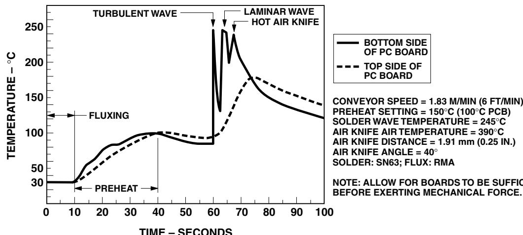
Figure 10. Recommended wave soldering profile
