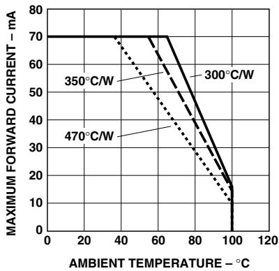
**Figure 5a. Maximum forward current vs. ambient temperature, derated based on  $T_{j\max} = 110^\circ\text{C}$  (AllnGaP)**
