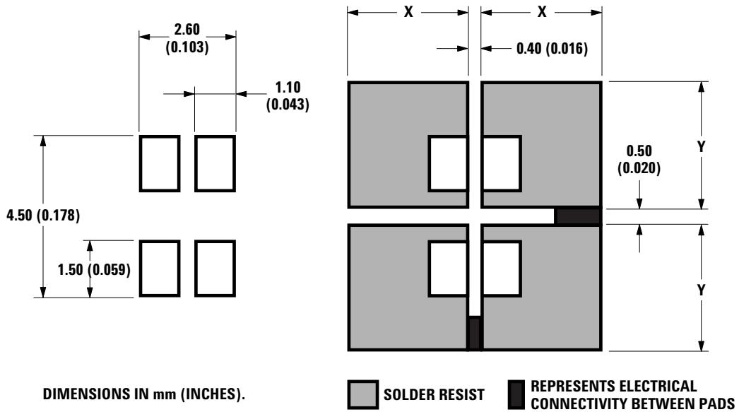
Figure 8a. Recommended soldering pad pattern
