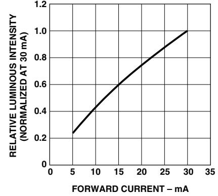
**Figure 4. Relative intensity vs. forward current
