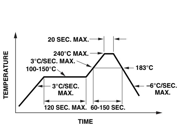
Figure 9a. Recommended SnPb reflow soldering profile
