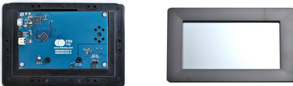
Figure 3-3 - VM800BU module profile 5" display version
