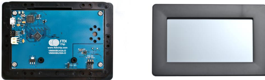
Figure 3-2 - VM800BU module profile 4.3" display version
