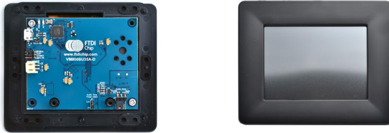
Figure 3-1 - VM800BU module profile 3.5" display version
