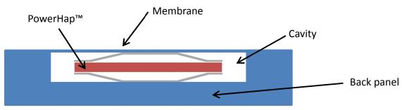
In this case the PowerHap actuator is clamped between a thin, flexible membrane and a rigid back panel. By applying a voltage, the actuator elongates and consequently deforms the membrane. In principle the membrane can be out of any material, but it may be necessary to tune the thickness. While the membrane needs to be as flexible as possible to maximize the haptic feedback felt by the user, it needs to be also stiff enough to properly clamp the actuator.
