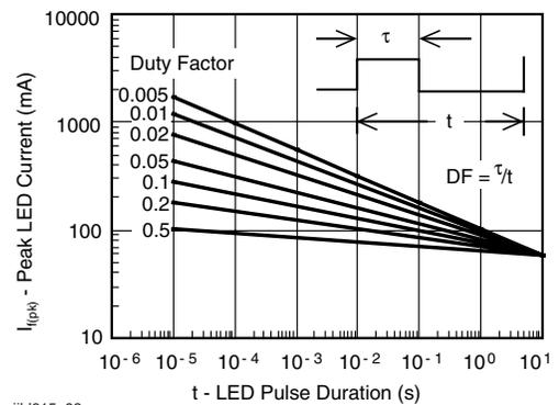
Fig. 8 - Peak LED Current vs. Pulse Duration,  $\tau$
