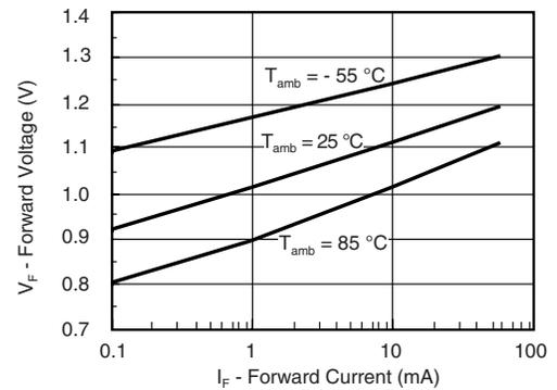
Fig. 7 - Forward Voltage vs. Forward Current
