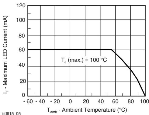
Fig. 5 - Maximum LED Current vs. Ambient Temperature
