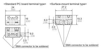
Material: Glass PTFE (Double sided, Through hole) R-4737 (Panasonic Corporation) Thickness: t = 0.8mm .031inch Copper thickness: 18µm
