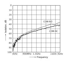
1-(2). High frequency characteristics (Impedance 75Ω) (Standard PC board terminal)
