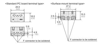
Material: Glass PTFE (Double sided, Through hole) R-4737 (Panasonic Corporation) Thickness: t = 0.8mm .031inch Copper thickness: 18µm
