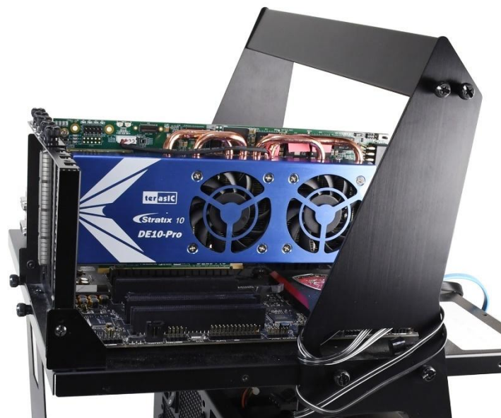
Figure 8-4 FPGA board installation on PC
