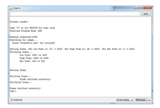
If you keep getting "Failed to verify fuses" while trying to restore the bootloader on a 3.3V Trinket using a Duemilanove. Try connecting 5V to the 3V pin on the Trinket, not VBAT+. Make sure USB is not plugged into the Trinket when you do this. Its a bit of a hack but may help!
