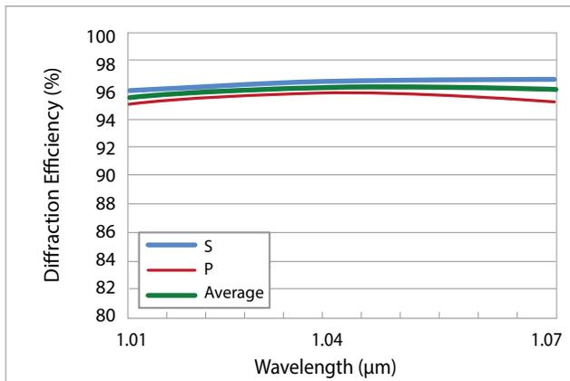
Typical absolute diffraction efficiency at AOI 31.3° \*
