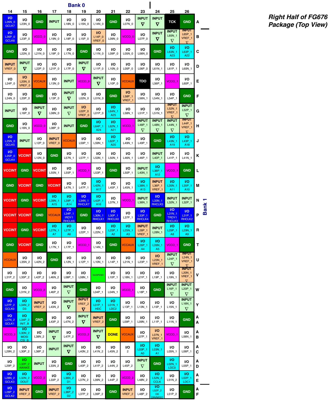
**Figure 17: FG676 Package Footprint for XC3SD1800A FPGA (Top View–Right Half)**
