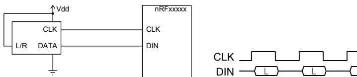
Figure 124: Example of a single PDM microphone, wired as left
