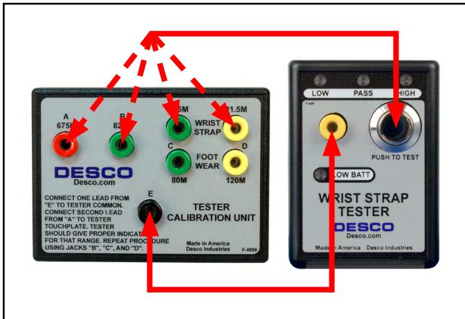
Figure 3. Verifying the calibration of the Wrist Strap Tester
