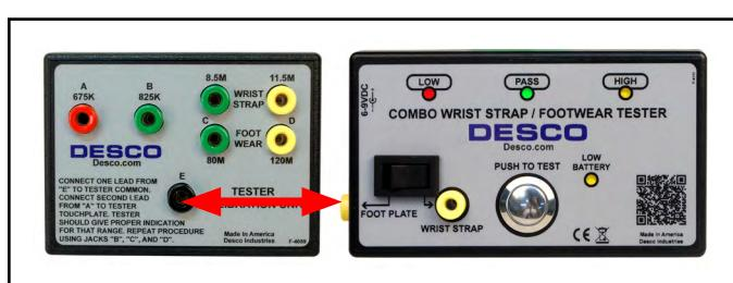
Figure 6. Connecting the test lead from banana jack "E" on the Calibration Unit to the FOOT PLATE banana jack on the Combo Tester
