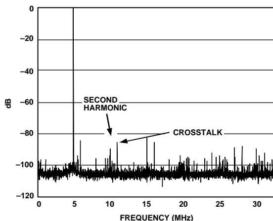
Figure 6. Single-Tone FFT of Channel A Digitizing  $f_{IN} = 70$  MHz
