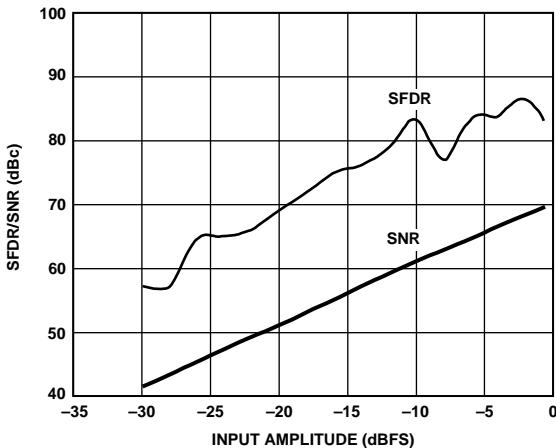
Figure 11. AD9238-65 Single-Tone SNR/SFDR vs. AIN with  $f_{IN} = 32.5\text{ MHz}$
