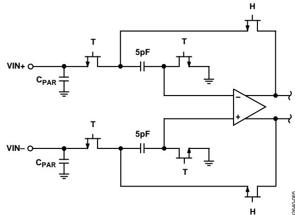
Figure 32. Switched-Capacitor Input
