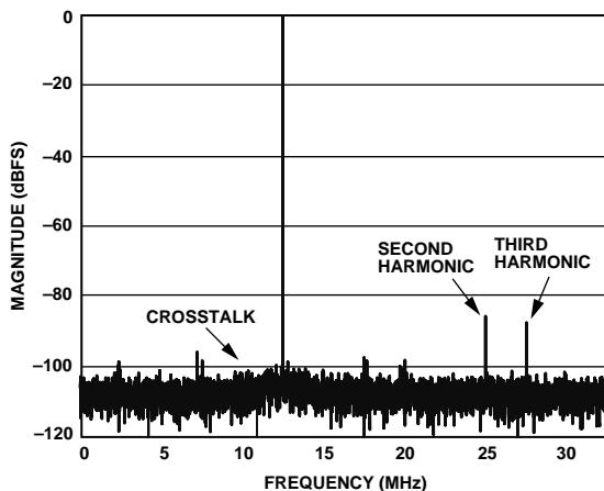
Figure 5. Single-Tone FFT of Channel A Digitizing  $f_{IN} = 12.5$  MHz
