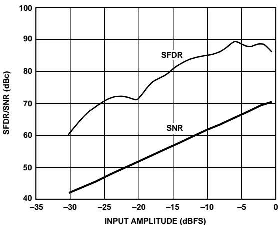
Figure 13. AD9238-20 Single-Tone SNR/SFDR vs. AIN with  $f_{IN} = 10\text{ MHz}$
