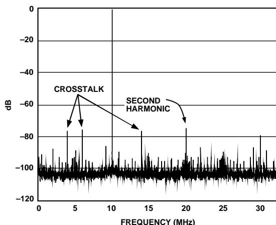
Figure 7. Single-Tone FFT of Channel A Digitizing  $f_{IN} = 120$  MHz
