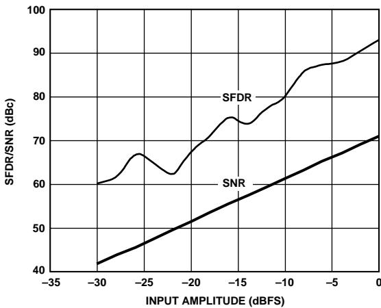
Figure 12. AD9238-40 Single-Tone SNR/SFDR vs. AIN with  $f_{IN} = 20\text{ MHz}$
