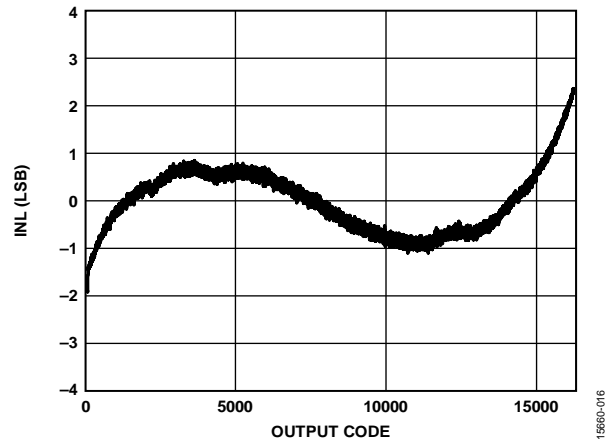
Figure 43. INL, f_{IN} = 10.3\text{ MHz}
