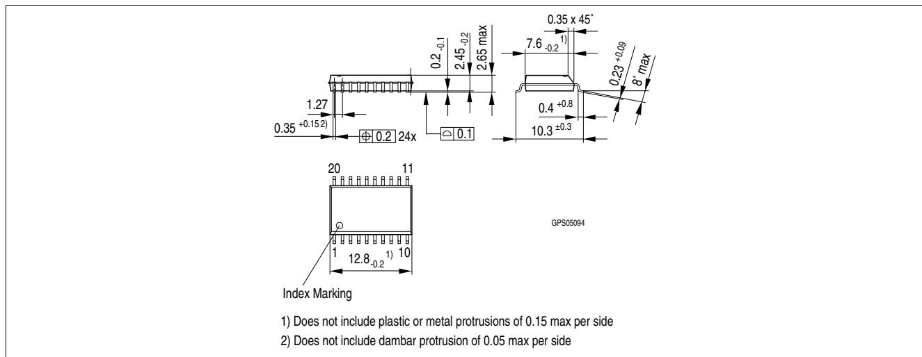
**Figure 1** PG-DSO-20 (Plastic Dual Small Outline Package) (RoHS-compliant)
