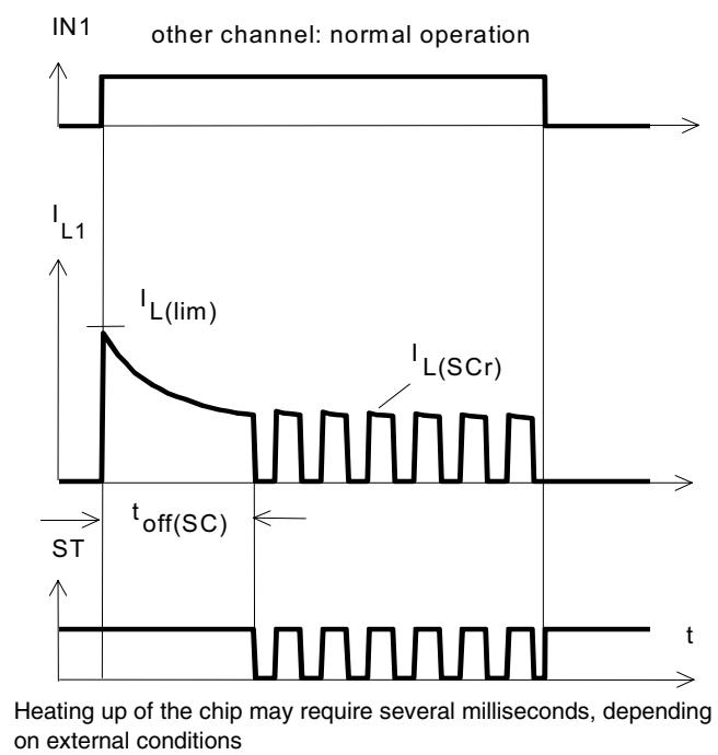
**Figure 3b:** Turn on into short circuit:
