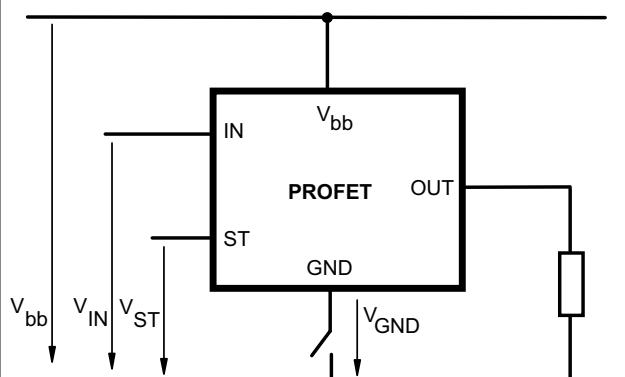
Any kind of load. In case of IN=high is  $V_{OUT} \approx V_{IN} - V_{IN(T+)}$ . Due to  $V_{GND} > 0$ , no  $V_{ST} = \text{low}$  signal available.
