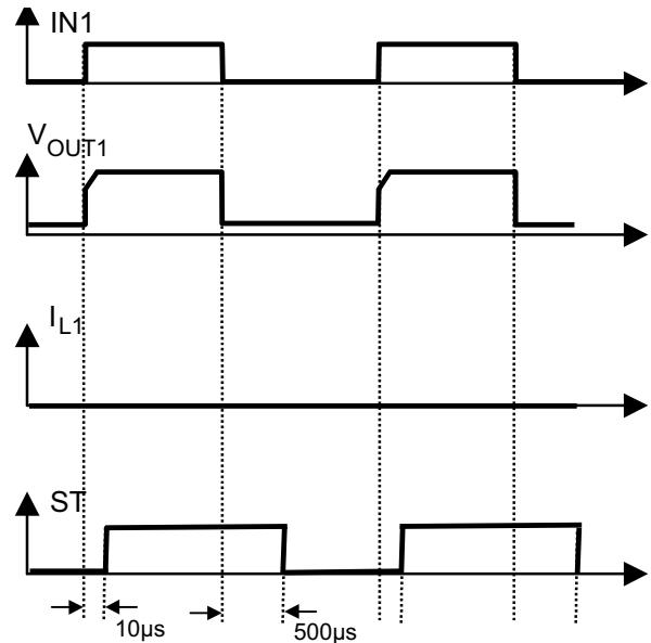
**Figure 6a:** Status change after, turn on/off to overtemperature
