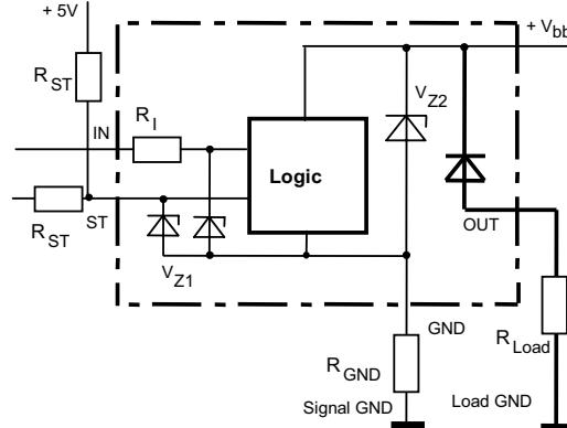
$V_{Z1} = 6.1$  V typ.,  $V_{Z2} = 47$  V typ.,  $R_{GND} = 150 \Omega$ ,  $R_{ST} = 15 \text{ k}\Omega$ ,  $R_I = 3.5 \text{ k}\Omega$  typ.
