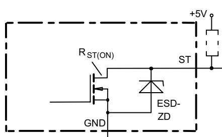
ESD-Zener diode: 6.1 V typ., max 0.3 mA;  $R_{ST(ON)} < 375 \Omega$  at 1.6 mA. The use of ESD zener diodes as voltage clamp at DC conditions is not recommended.
